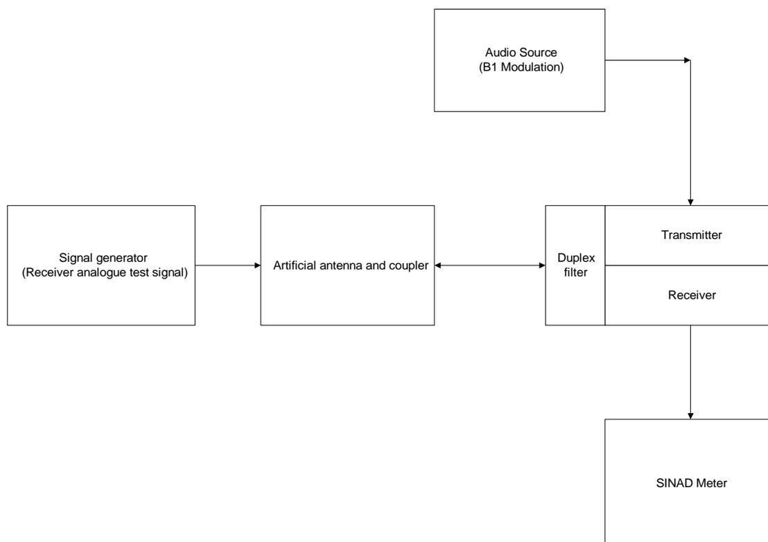
**Figure 6: Measurement arrangement**
