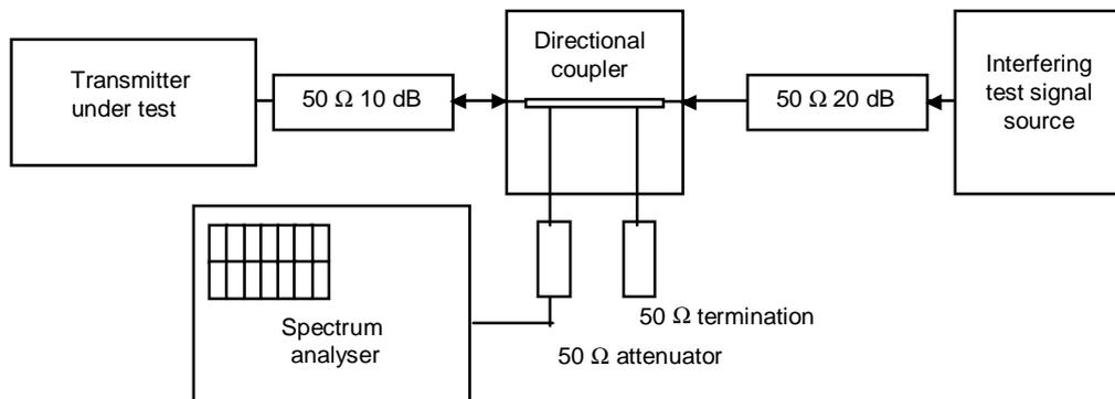
**Figure 3: Measurement arrangement**
