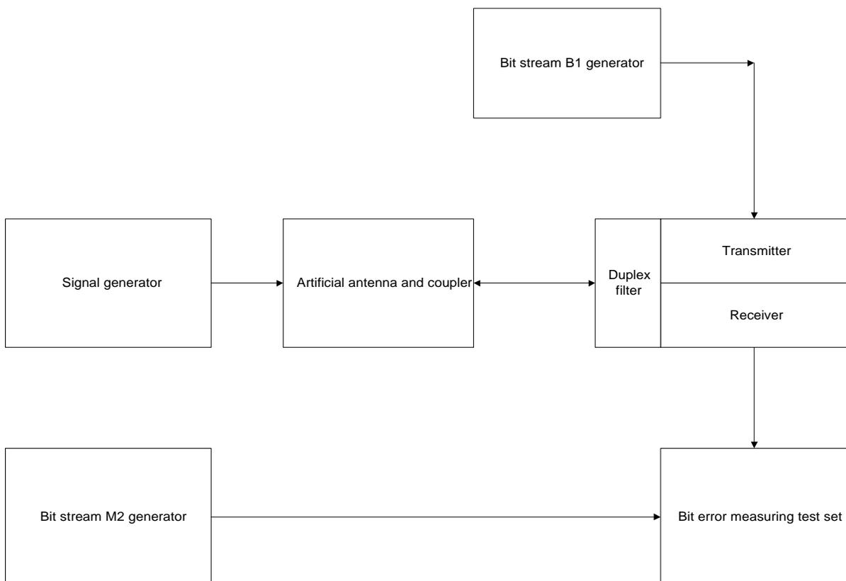
**Figure 16: Measurement arrangement for digital equipment (messages) having a duplex filter**
