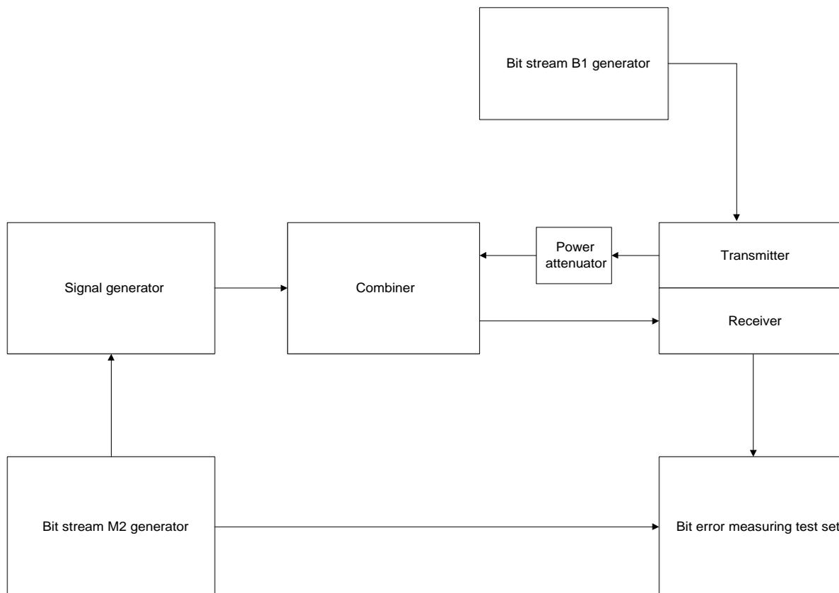
**Figure 9: Measurement arrangement**
