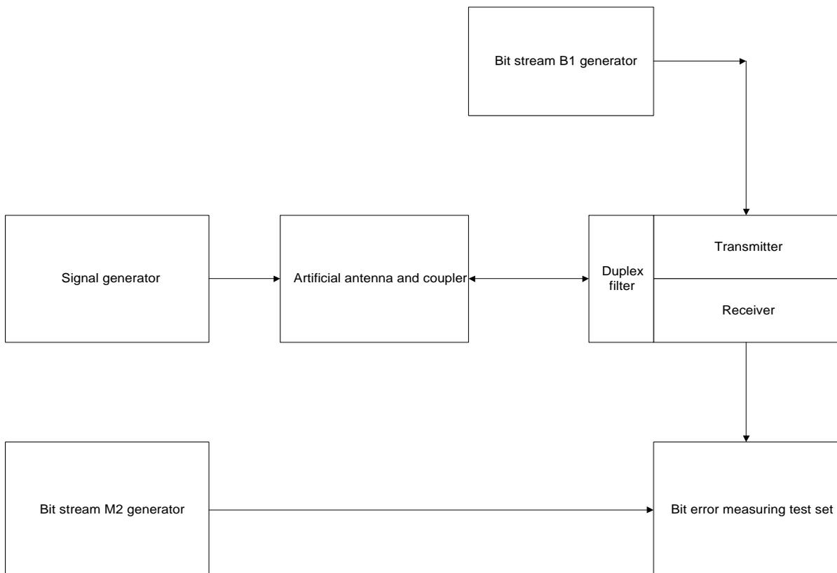
**Figure 14: Measurement arrangement for digital equipment (continuous bit streams) having a duplex filter**
