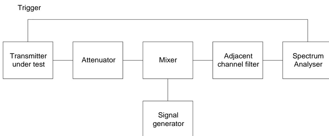
**Figure 4: Transient power measuring device measurement arrangement**
