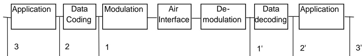
**Figure 2: Test points for bit stream measurements**
