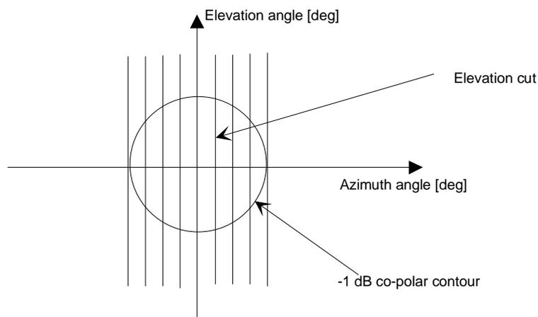
**Figure 4: Measurement of the antenna XPD in the -1 dB co-polar contour**
