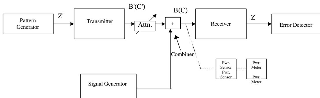
**Figure 15: Test configuration for CW spurious interference**
