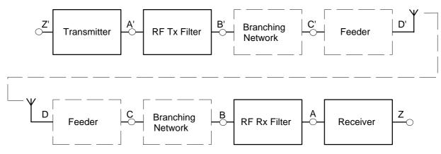
Figure 2: RF system block diagram
