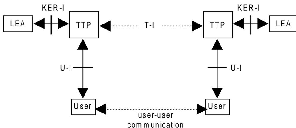
Figure 4: General end-to-end encryption configuration with key escrow
