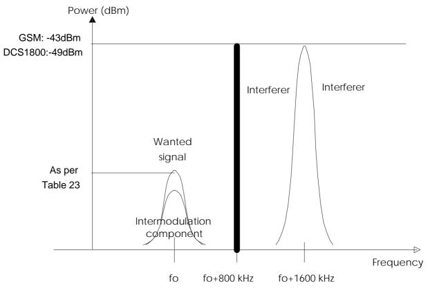
Figure 6: Example of RX intermodulation rejection
