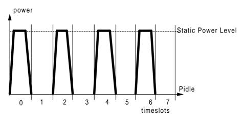
Figure 4: Power/time slot configuration (no RF power control)
