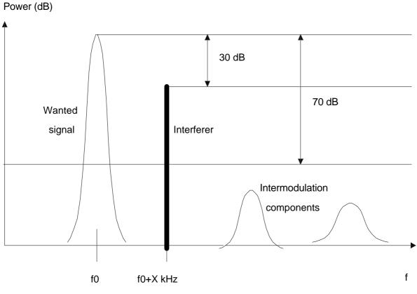
Figure 5: Example of TX intermodulation attenuation
