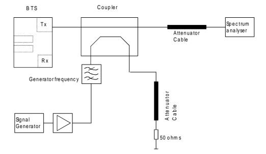
Figure B.2: Test set-up for Intermodulation Attenuation (6.7.) outside RX-Band
