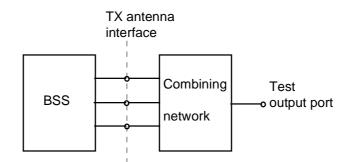
Figure 1b. Transmitter test setup
