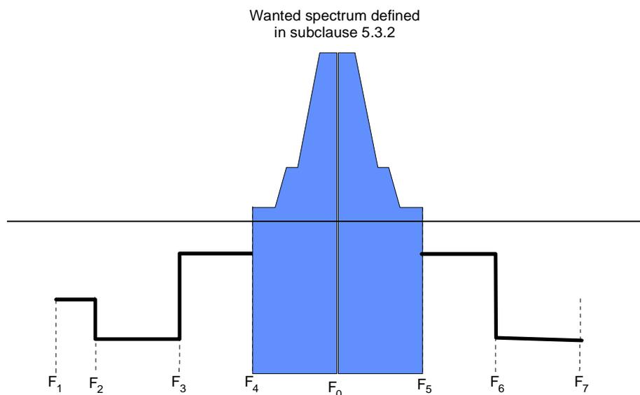
**Figure 4: Spectrum mask for transmitter spurious emissions****Table 4.3: Frequency breakpoints for spurious emissions in figure 4**
