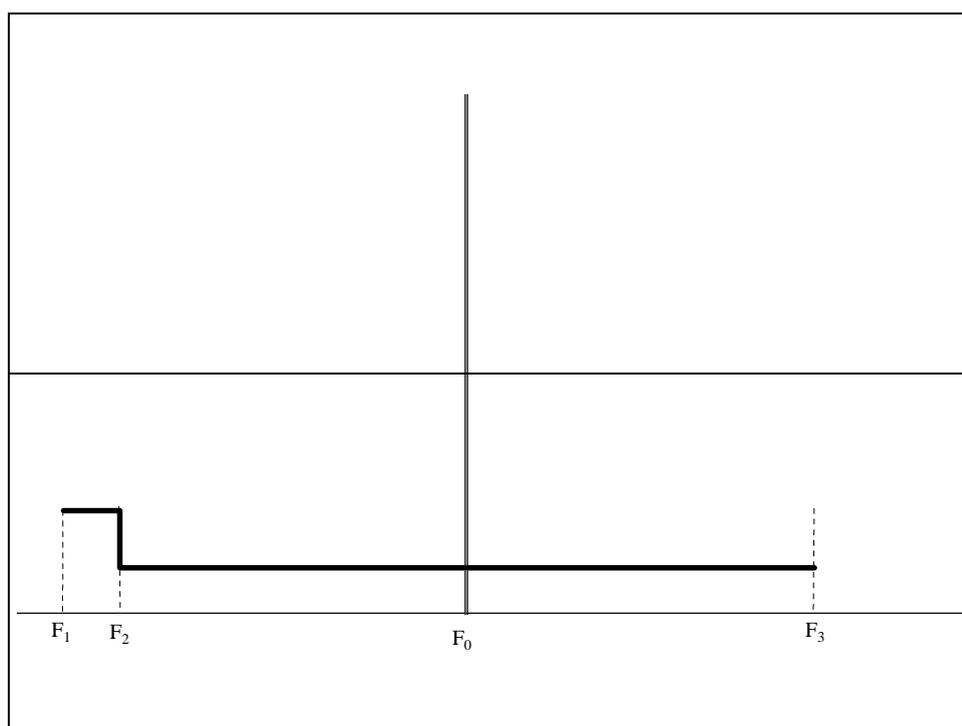
**Figure 5: Spectrum mask for receiver spurious emissions**
