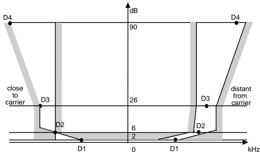
Figure B.1: IF filter characteristics
