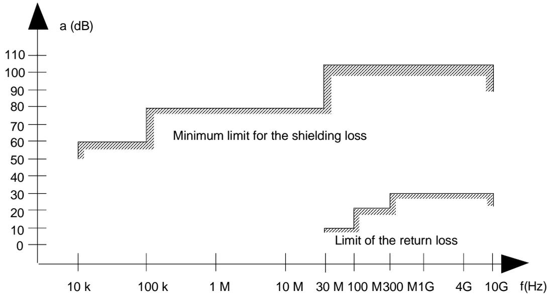
Figure C.3: Specifications for shielding and reflections
