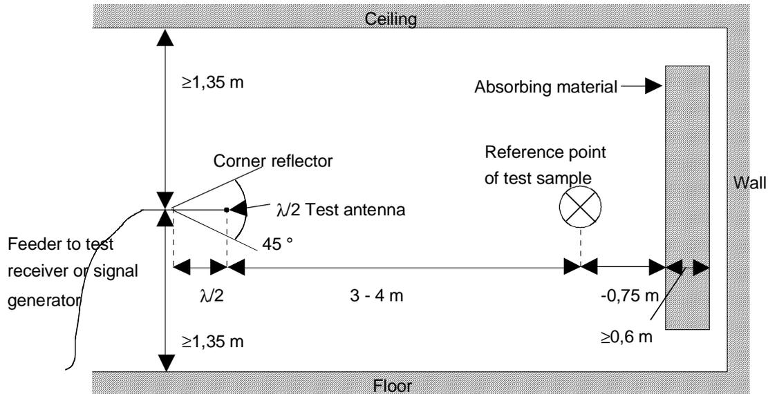
Figure C.2: Indoor site arrangement (shown for horizontal polarization)
