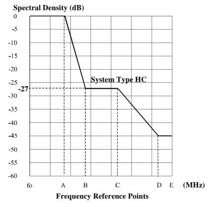
Figure 5: Power spectrum masks for system type HC (fo = actual carrier frequency)
