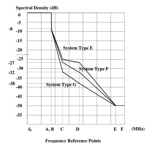
Figure 4: Power spectrum masks for system type E, F and G (fo = actual carrier frequency)
