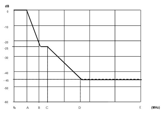
Figure 3: Power spectrum mask (fo = actual carrier frequency)
