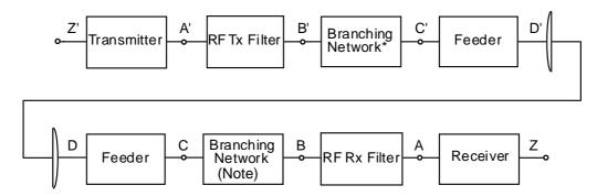
NOTE: Points B and C and B' and C' will coincide if branching networks are not used.
