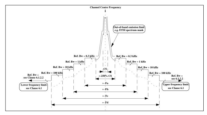
NOTE: ± Fd frequency steps are not applicable if lower than 1 GHz
