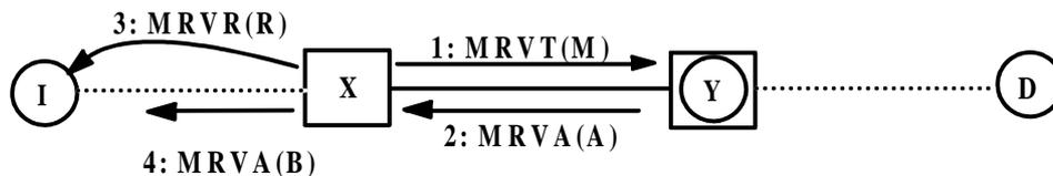
Consider the preceding diagram. I is an MRV Test initiator, X an STP which apparently has a route to the test destination D through Y. I is unknown to Y.
