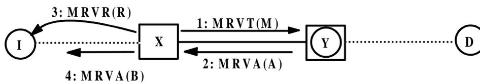
Consider the preceding diagram. I is an MRV Test initiator, X an STP which apparently has a route to the test destination D through Y. I is unknown to Y.
