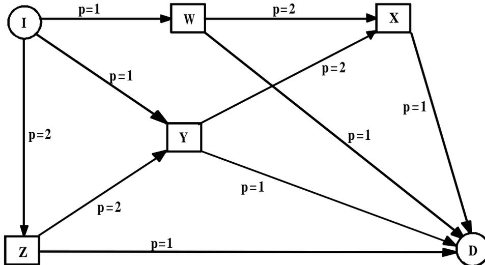
Here, the test initiator is denoted by I, the test destination by D, and W, X, Y and Z denote intermediate STPs. All the routes defined in the routing tables are shown, and their directions. The priorities of the routes to the test destination are also shown (thus e.g. the route WXD, forming part of the route IWXD, has priority 2 at W. The linksets IW and IY have equal first priority, and form a combined linkset to D). Assume for the purposes of this example that all routes to D are available.
