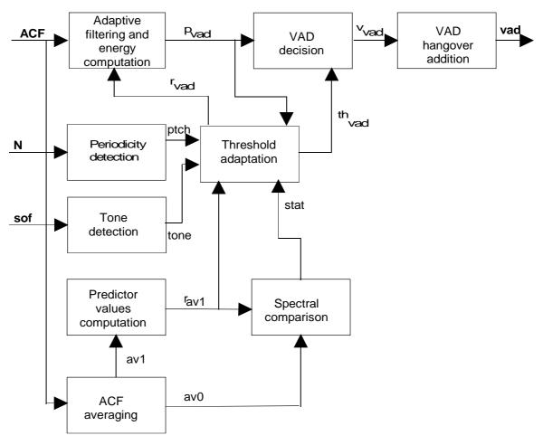
Figure 2.1: Functional block diagram of the VAD
