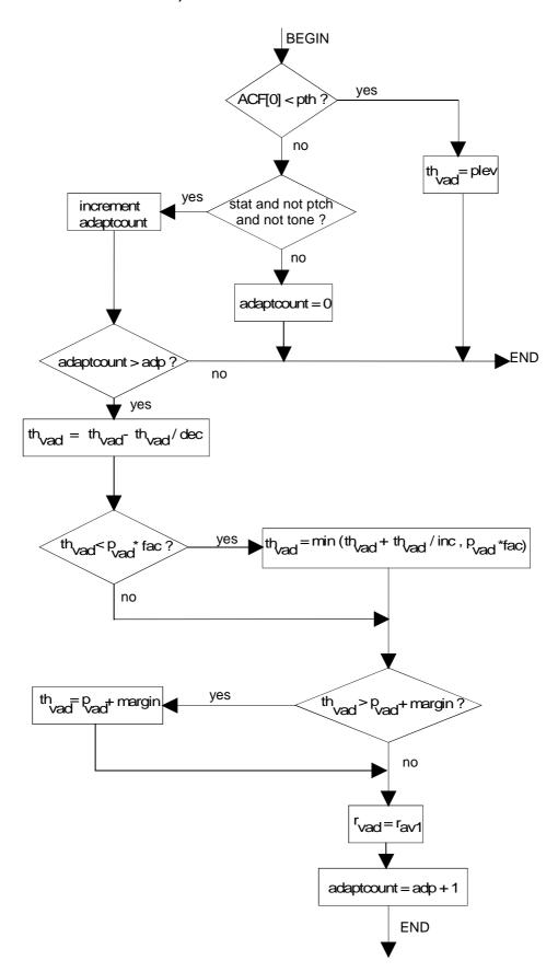
Figure 2.2: Flow diagram for threshold adaptation
