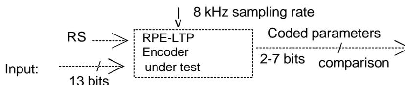
Figure 6.1: Configuration 1: RPE-LTP encoder under test
