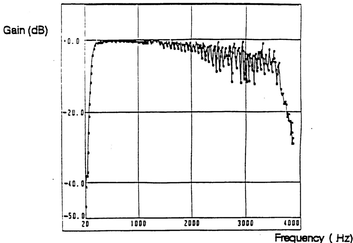
Figure A.1.5: Frequency response for RPE-LTP codec
