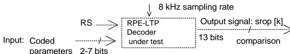
Figure 6.2: Configuration 2: RPE-LTP decoder under test
