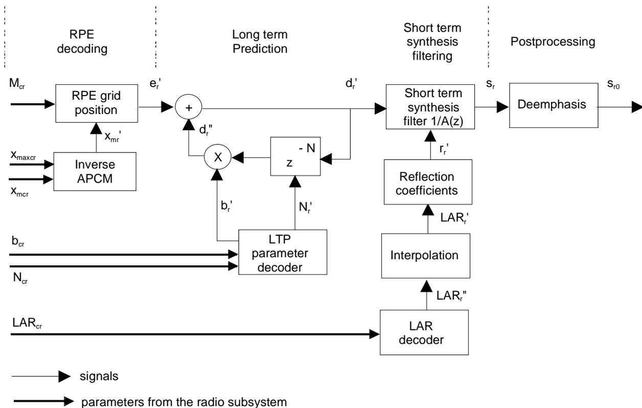
Figure 3.4: Block diagram of the RPE-LTP decoder
