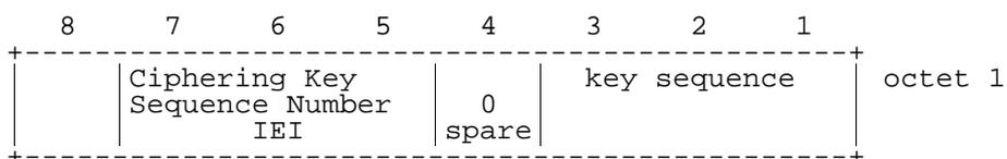
**Figure 10.5.2/GSM 04.08: Ciphering Key Sequence Number information element**
