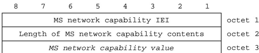
Figure 10.5.128/GSM 04.08: MS network capability information element
