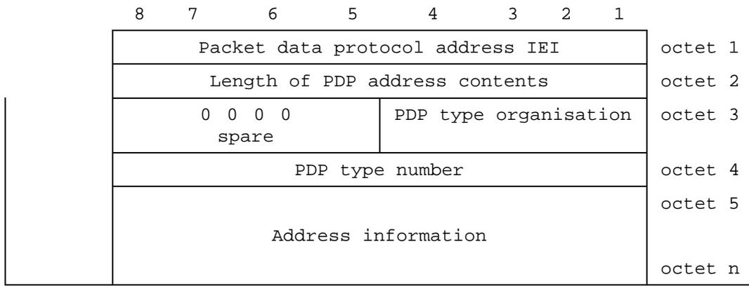
Figure 10.5.137/GSM 04.08: *Packet data protocol address information element*
