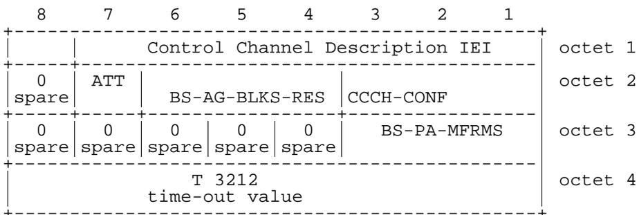
**Figure 10.5.33/GSM 04.08: Control Channel Description information element**
