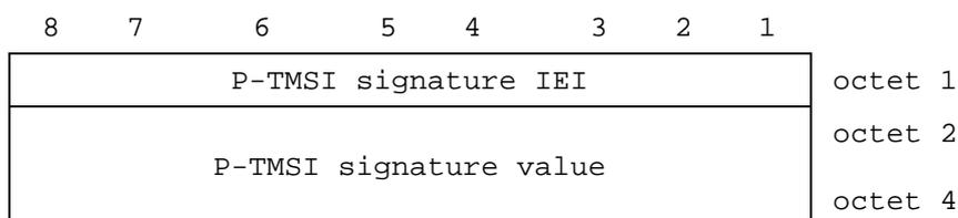
**Figure 10.5.124/GSM 04.08: P-TMSI signature information element**
