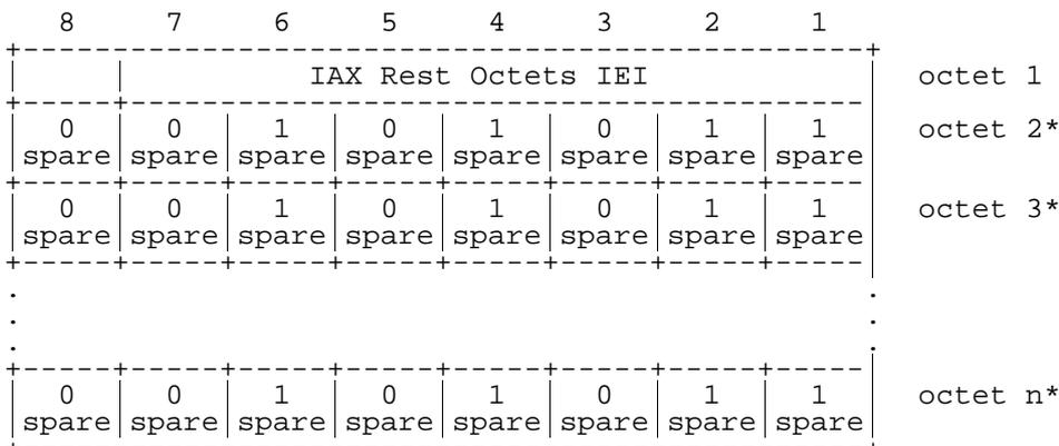
**Figure 10.5.45/GSM 04.08: IAX Rest Octets information element**
