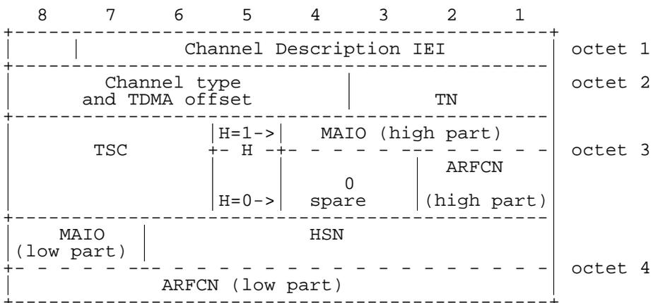
**Figure 10.5.26/GSM 04.08: Channel Description 2 information element**
