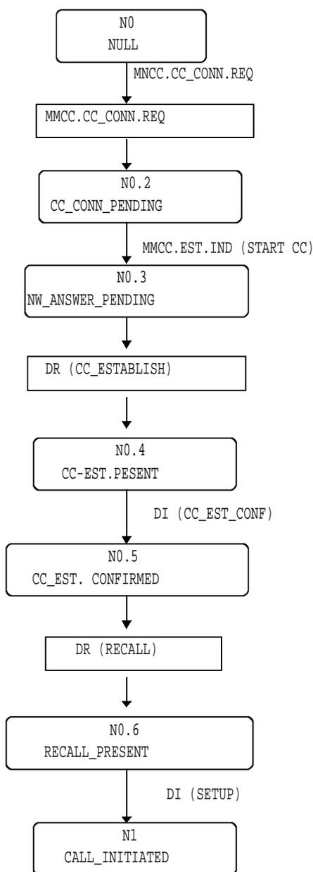
Figure 5.1b.1/GSM 04.08: Overview call control protocol/Network side, extension:
