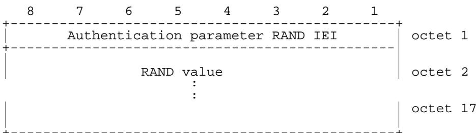
**Figure 10.5.75/GSM 04.08: Authentication Parameter RAND information element**
