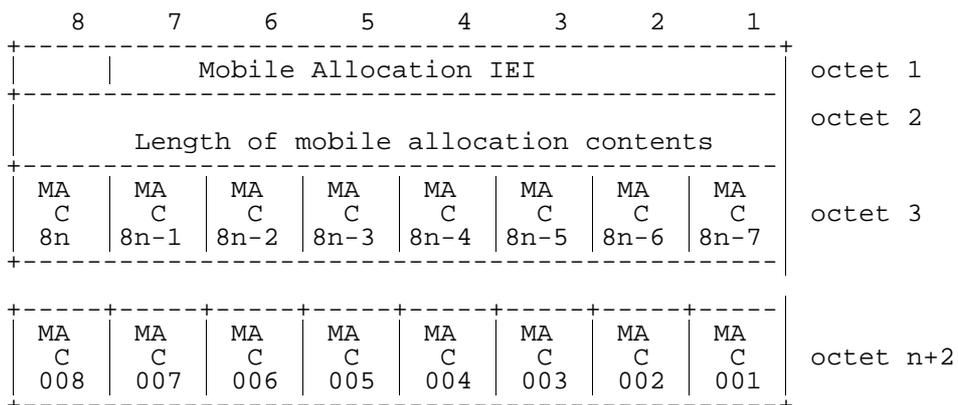
**Figure 10.5.49/GSM 04.08: Mobile Allocation information element**
