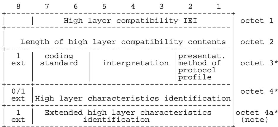
Figure 10.5.102/GSM 04.08: High layer compatibility information element
