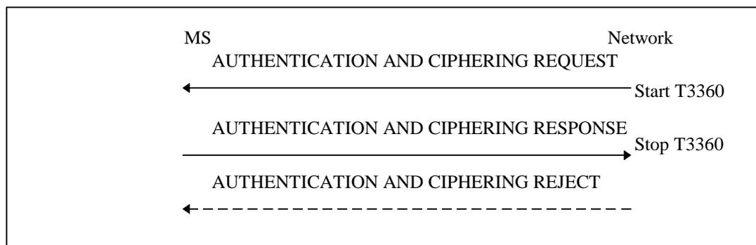
**Figure 4.7.7/1 GSM 04.08: Authentication and ciphering procedure**
