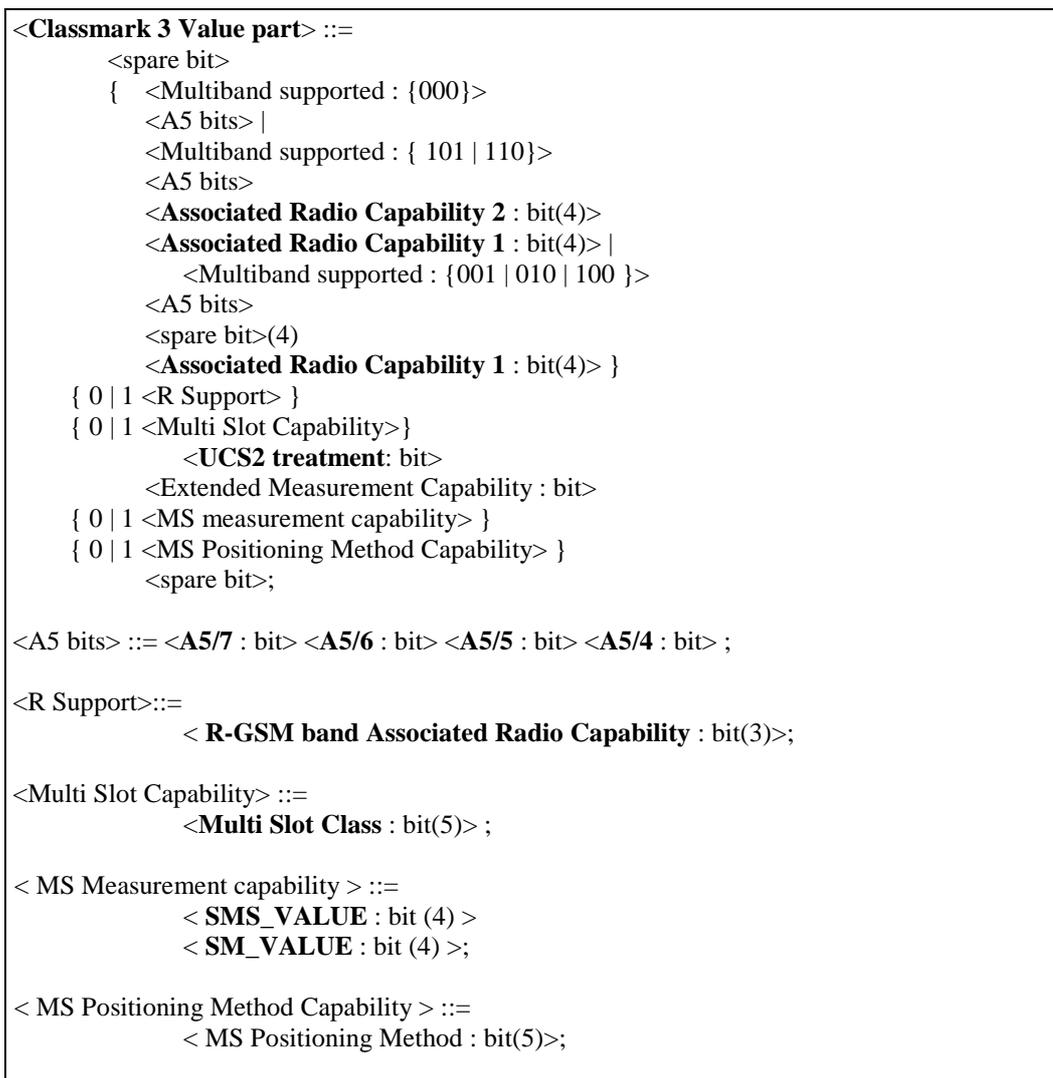
Figure 10.5.7/GSM 04.08: *Mobile Station Classmark 3* information element
