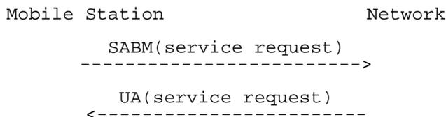
**Figure 7.4/GSM 04.08: Service request and contention resolution**
