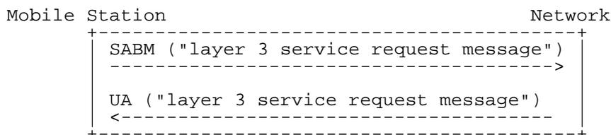
Figure 3.1/GSM 04.08 Service request and contention resolution
