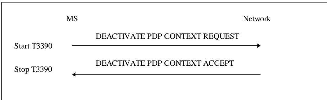
Figure 6.6/GSM 04.08: MS initiated PDP context deactivation procedure
