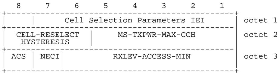
Figure 10.5.23/GSM 04.08: *Cell Selection Parameters* information element
