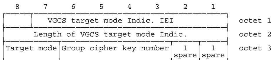
**Figure 10.5.71/GSM 04.08: VGCS target mode Indication information element**
