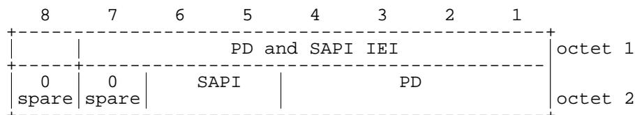
**Figure 10.5.10/GSM 04.08: PD and SAPI information element**
