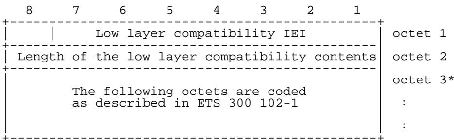
Figure 10.5.104/GSM 04.08: Low layer compatibility information element
