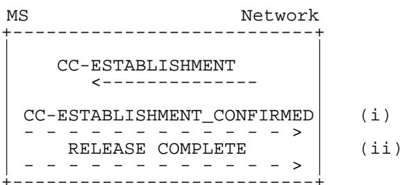
Figure 5.7a/GSM 04.08: Call initiation and possible subsequent responses
