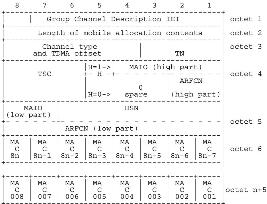
Figure 10.5.41/GSM 04.08: *Group Channel Description* information element
