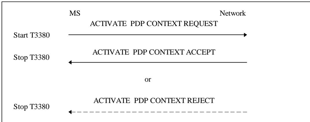
Figure 6.3/GSM 04.08: MS initiated PDP context activation procedure
