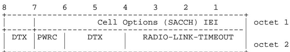
Figure 10.5.22/GSM 04.08: Cell Options (SACCH) information element
