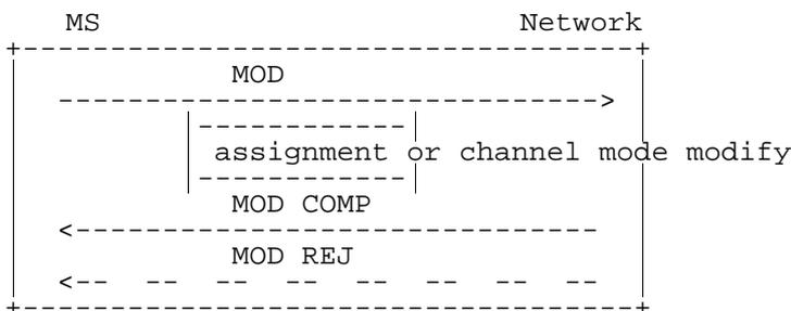
Figure 5.10a/GSM 04.08 In-call modification sequence initiated by MS
