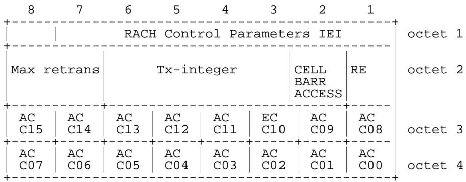
Figure 10.5.60/GSM 04.08: RACH Control Parameters information element
