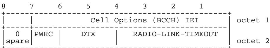
Figure 10.5.21/GSM 04.08: Cell Options (BCCH) information element
