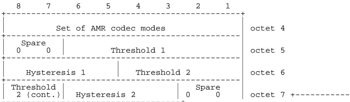
Figure 10.5.2.47c/GSM 04.08: Parameters for multirate speech field for the MR version 1 when a set of three codec modes is chosen
