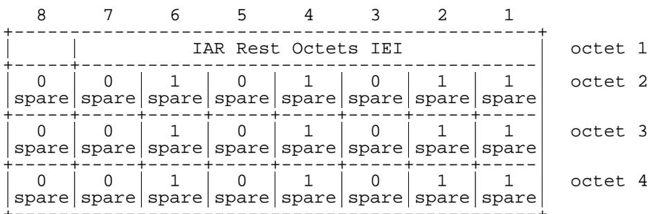
**Figure 10.5.44/GSM 04.08: IAR Rest Octets information element**
