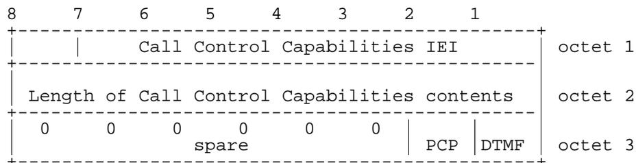
**Figure 10.5.89/GSM 04.08: Call Control Capabilities information element**
