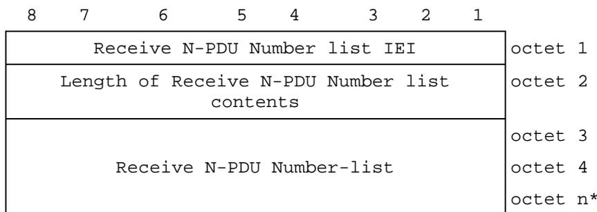
Figure 10.5.127/GSM 04.08: Receive N-PDU Number list information element
