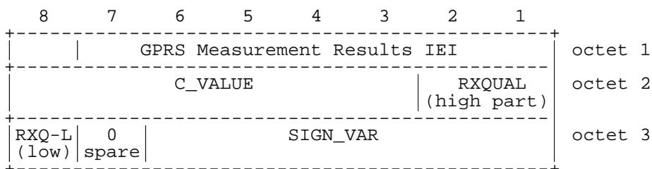
**Figure 10.5.48/GSM 04.08: GPRS Measurement Results information element**
