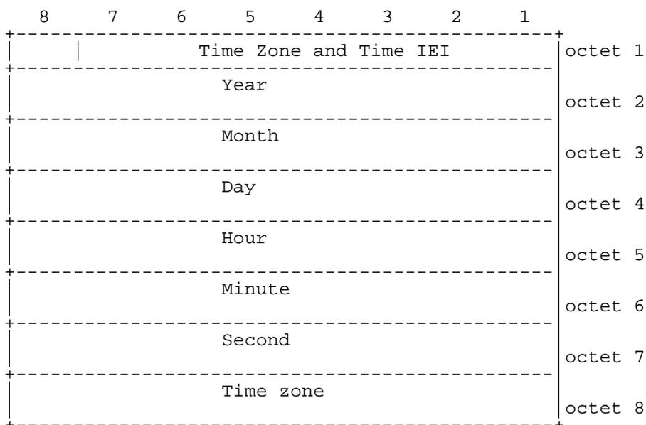
Figure 10.5.84/GSM 04.08: *Time Zone and Time* information element
