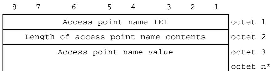
**Figure 10.5.134/GSM 04.08: Access point name information element**
