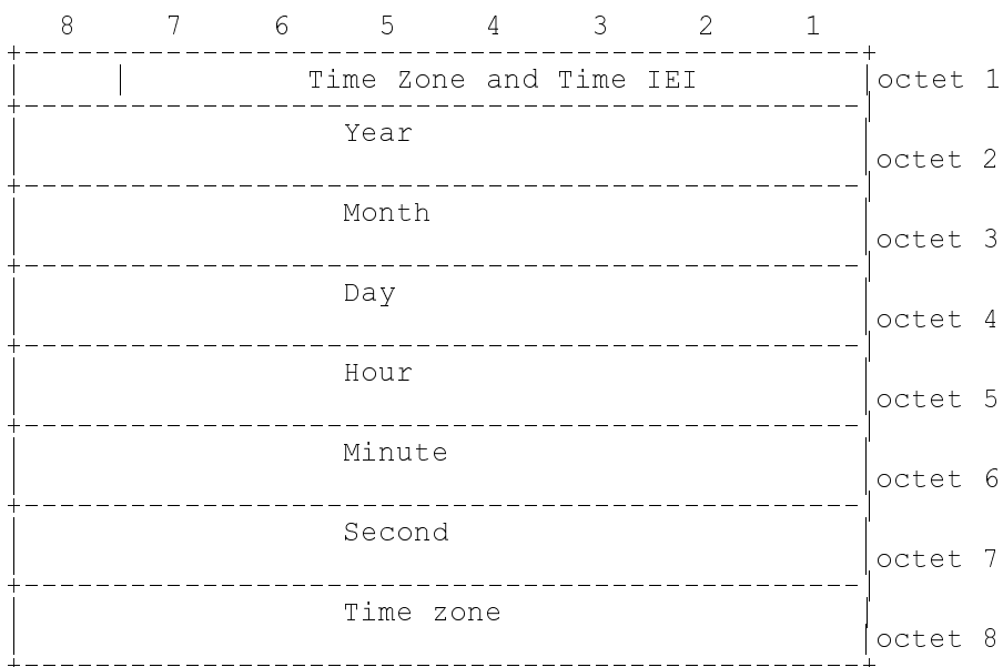
Figure 10.5.84/GSM 04.08 Time Zone and Time information element
