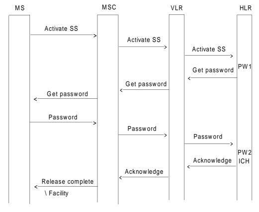
NOTE: SS indicates any of the protected supplementary services. PW1 and PW2 indicate password handling programs. ICH indicates interaction checks if necessary. Figure 3.6: Activation of protected supplementary service
