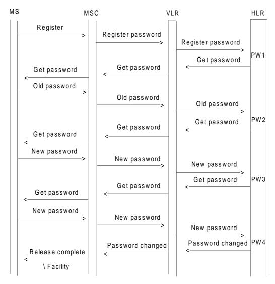
NOTE: PW1, PW2 and PW3 indicate password handling programs. Figure 3.5: Registration of a new password
