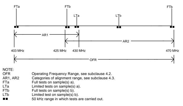
This example requires a minimum of two test samples and a maximum of five test samples to cover the operating frequency range.
