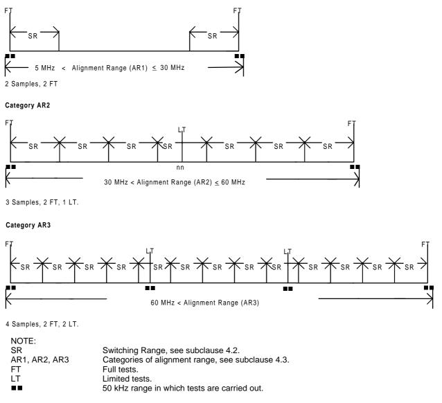
Figure A.2: Tests on equipment having switching ranges that are subsets of their alignment range
