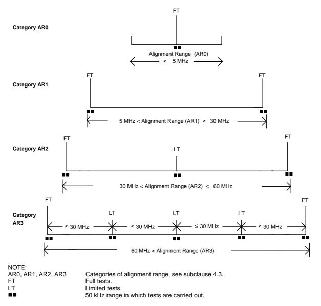
Figure A.1: Tests on a single sample for equipment that has a switching range equal to its alignment range
