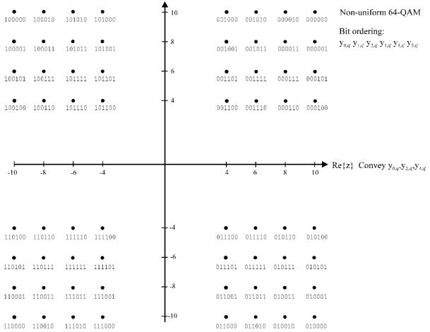
Figure 9c: Non-uniform 16-QAM and 64-QAM mappings with  $\alpha = 4$
