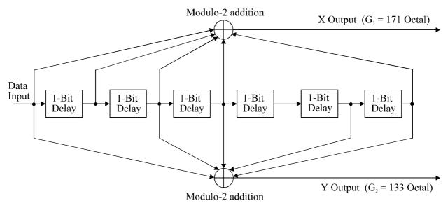
Figure 5: The mother convolutional code of rate 1/2
