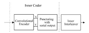
Figure 6: Inner coding and interleaving
