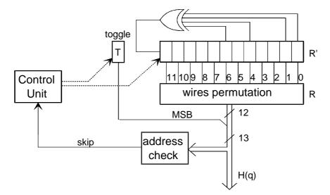
Figure 8b: Symbol interleaver address generation scheme for the 8K mode
