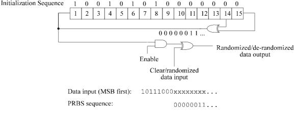
Figure 2: Scrambler/descrambler schematic diagram
