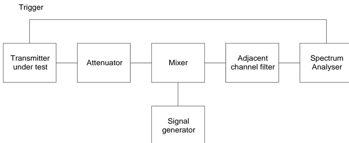
**Figure 5: Transient power measuring device measurement arrangement**
