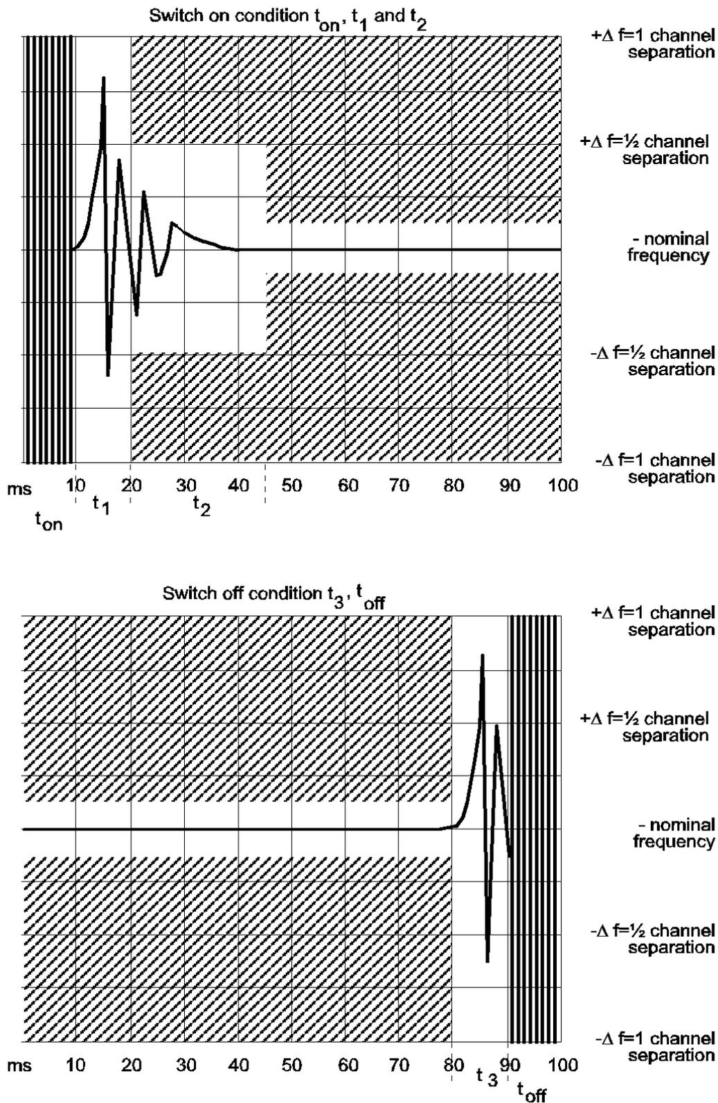
Figure 4: Frequency error - v - time
