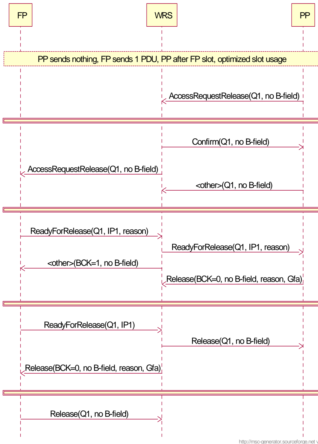
Figure 21: Single burst downlink, PP initiated - PP after FP slot - optimized slot usage
