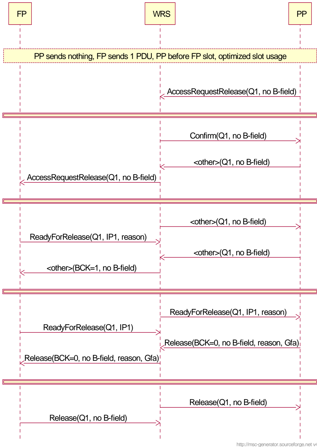
Figure 21a: Single burst downlink, PP initiated - PP before FP slot - optimal slot usage
