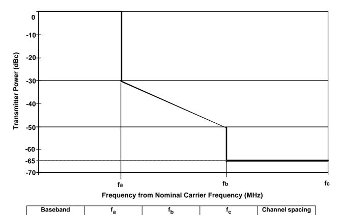
Figure 2a: Limits of spectral power density for video, standard frequency deviation
