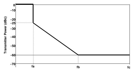
Frequency offset from Nominal Carrier Frequency (MHz)
