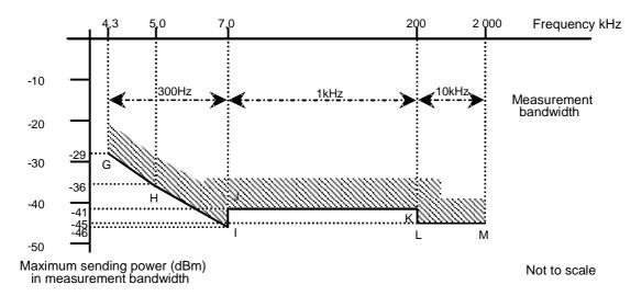
Figure 4: Maximum sending power above 4,3 kHz
