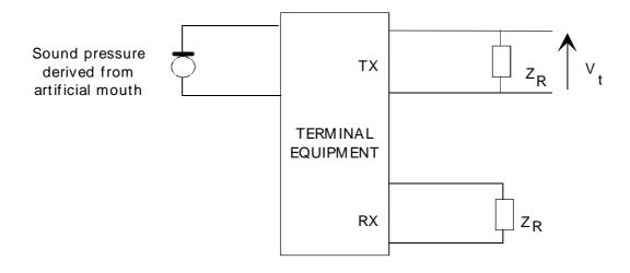
Figure A.3: Measurement of sending sensitivity
