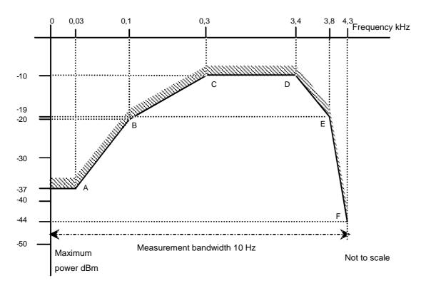
Figure 3: Maximum power in a 10 Hz bandwidth
