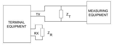
Figure A.7: Maximum sending power above 4,3 kHz
