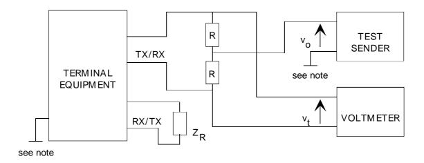
The resistors R shall be 300  $\Omega\pm1$  % and matched to better than 0,1 %. The test sender output impedance is not critical.
