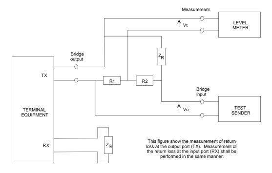
R1 = R2; between 100  $\Omega$  and 800  $\Omega$ , preferably 600  $\Omega$ , matched to better than 0,2 %. Test sender output impedance < 10  $\Omega$ .
