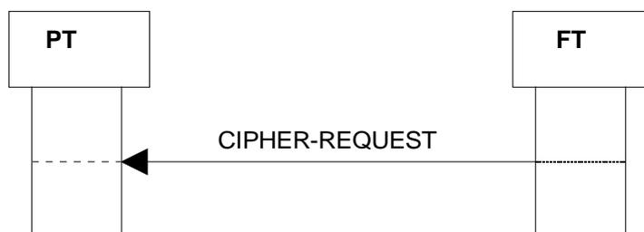
Figure 94: Cipher - switching initiated by FT
