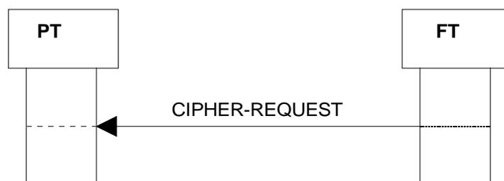
Figure 66: Cipher - switching initiated by FT
