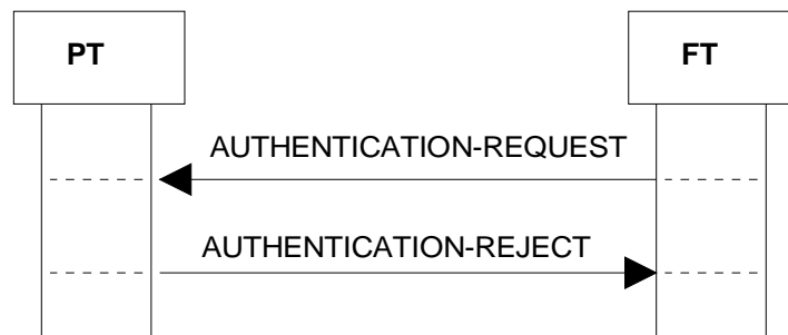
Figure 51: Authentication algorithm/key not supported by the PT
