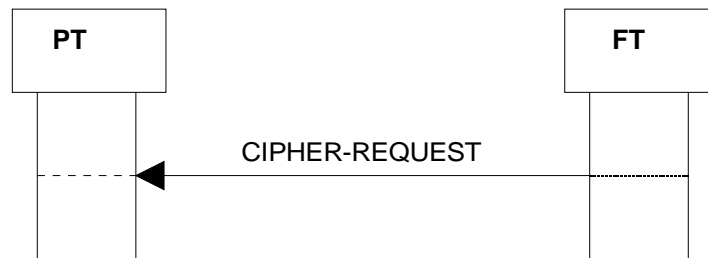
Figure 65: Cipher - switching initiated by FT
