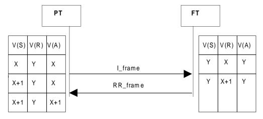
NOTE 1: During the calculation of the variable's values an assumption has been made that the I\_frame sent by PT is not used for acknowledgement of previous received I\_frames and is not a re-transmission.
