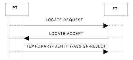
Figure 55: Rejection of identity assignment
