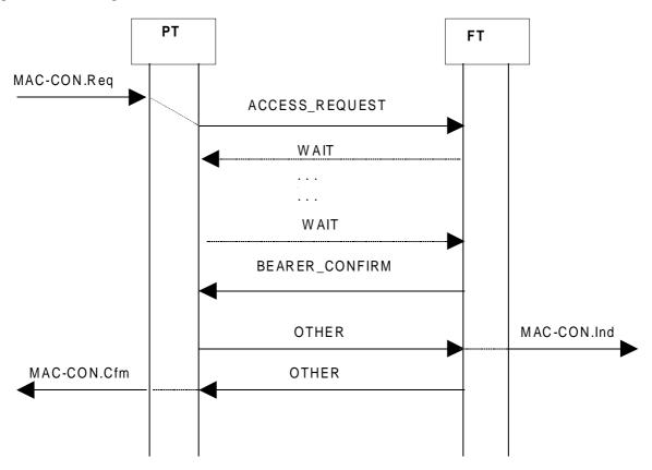
Figure 87: Setup of basic connection and bearer
