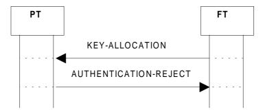
Figure 62: Allocation-type unacceptable for PT
