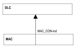
Figure 81: Establishment of a MAC connection receiving side
