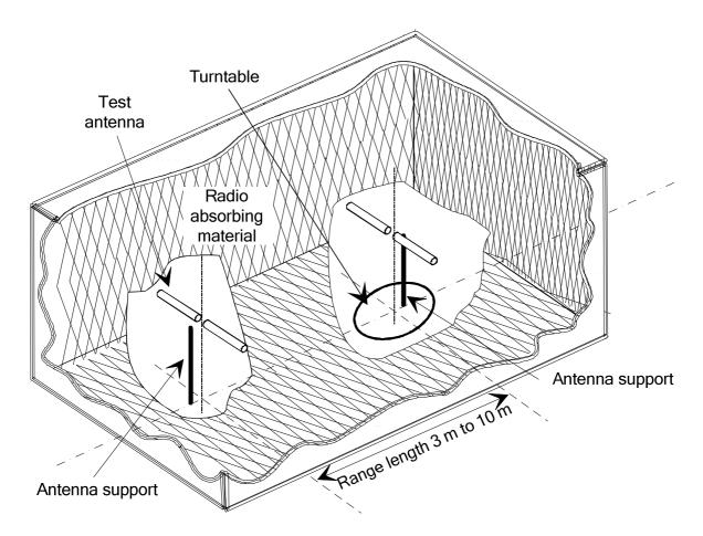
Figure A.1: A typical anechoic chamber
