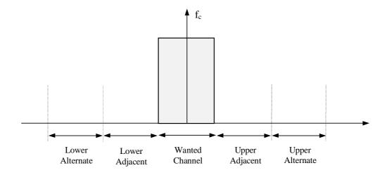
Figure 0: Adjacent and alternate channel definitions
