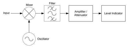
Figure B.1: Power measuring receiver
