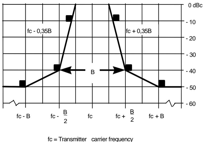
**Figure 6: Spectrum mask for analogue or digital Body Worn systems in all bands**
