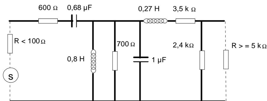
**Figure 2: Filter circuit**
