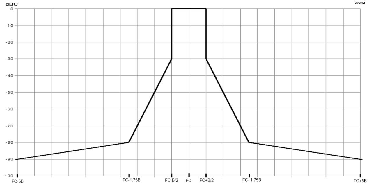
**Figure 4: Spectrum mask for digital systems below 2 GHz**
