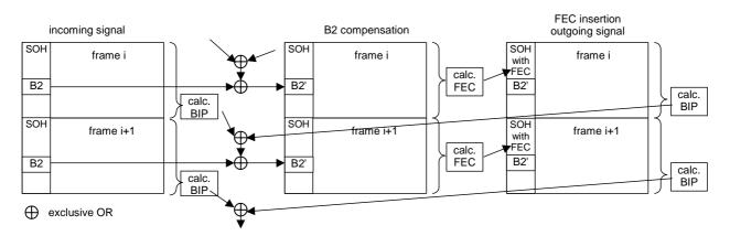
Figure 143: B2 compensation and FEC calculation
