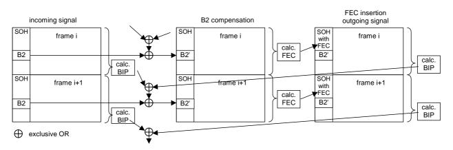
Figure 195: B2 compensation and FEC calculation
