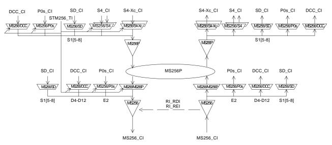
Figure 202: STM-256 Multiplex Section Linear Trail Protection Functions
