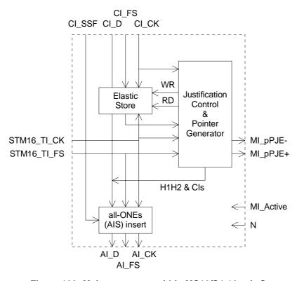
Figure 103: Main processes within MS16/S4-16c\_A\_So
