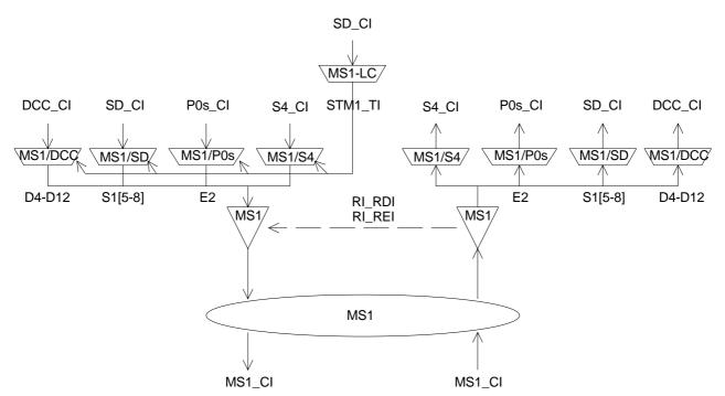
Figure 15: STM-1 Multiplex Section atomic functions
