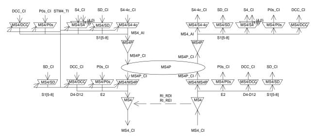
Figure 53: STM-4 Multiplex Section Linear Trail Protection Functions
