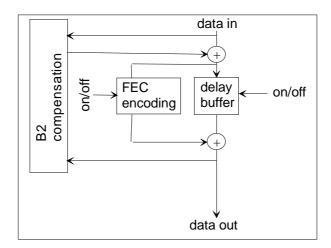
Figure 142: STM-64 FEC encoding process
