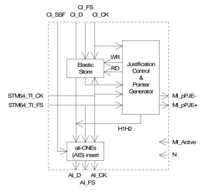
Figure 155: Main processes within MS64/S4\_A\_So
