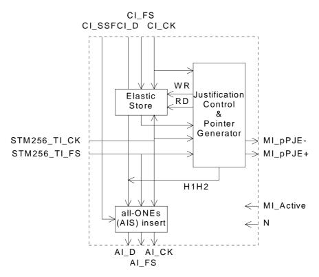
Figure 207: Main processes within MS256/S4\_A\_So
