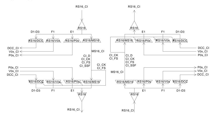
Figure B.1: STM-16 regenerator model (supporting DCC, OW, USR)
