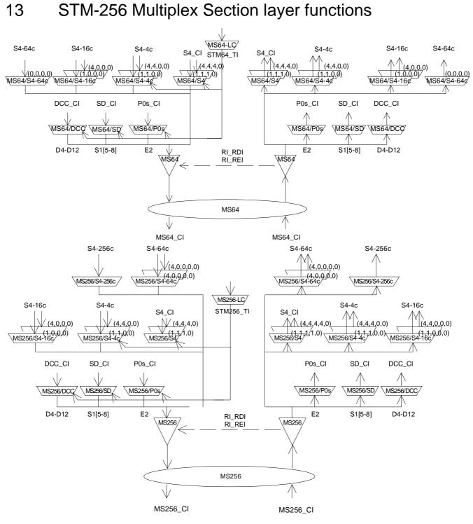
Figure 199: STM-256 Multiplex Section atomic functions
