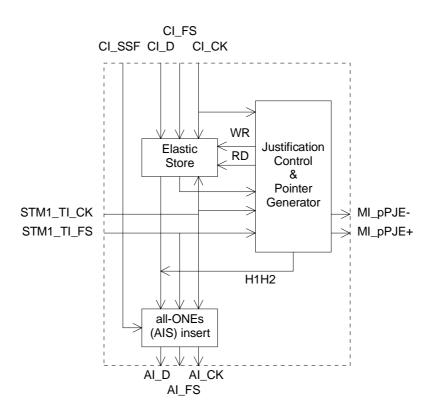
Figure 23: Main processes within MS1/S4\_A\_So
