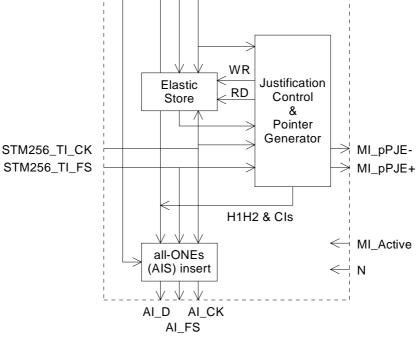
Figure 213: Main processes within MS256/S4-16c\_A\_So
