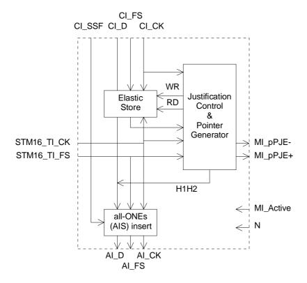
Figure 97: Main processes within MS16/S4\_A\_So
