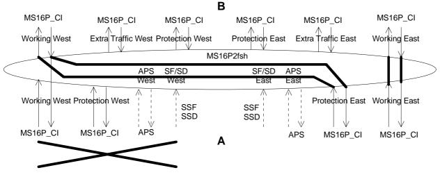
Figure 119: Matrix connections in a network element adjacent to a fault on its west side
