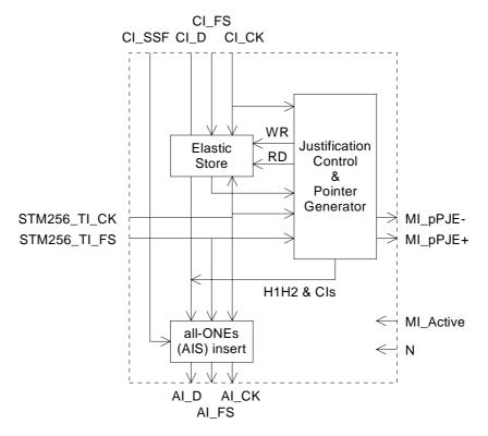
Figure 219: Main processes within MS256/S4-256c\_A\_So
