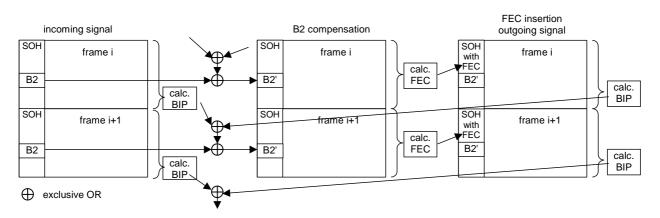
Figure E.5: B2 compensation and FEC calculation
