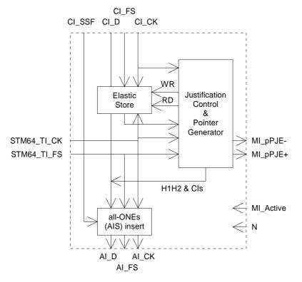
Figure 164: Main processes within MS64/S4-64c\_A\_So
