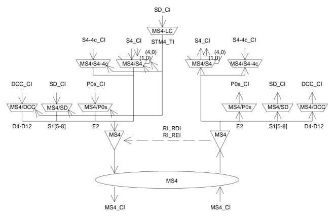
Figure 50: STM-4 Multiplex Section atomic functions
