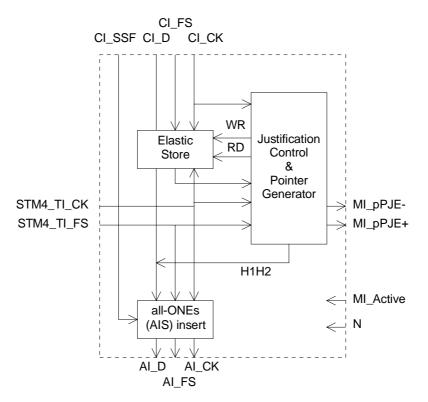
Figure 58: Main processes within MS4/S4\_A\_So
