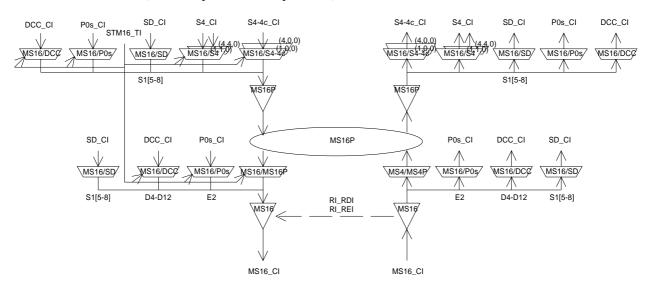
Figure 91: STM-16 Multiplex Section Linear Trail Protection Functions
