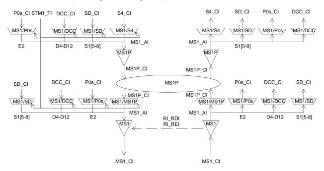
Figure 18: STM-1 Multiplex Section Linear Trail Protection Functions
