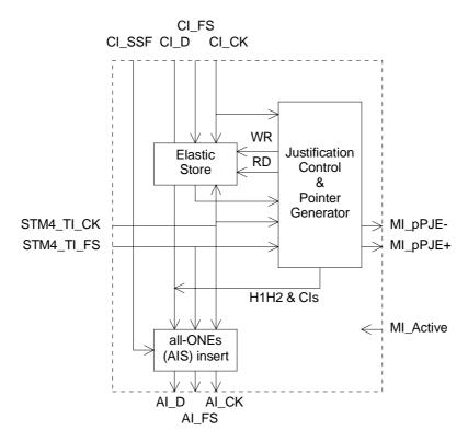
Figure 61: Main processes within MS4/S4-4c\_A\_So
