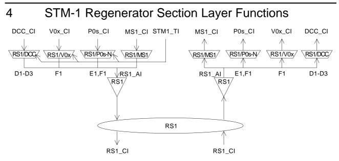
Figure 1: STM-1 Regenerator Section atomic functions
