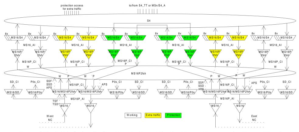
Figure 94: STM-16 Multiplex Section 2 fibre Shared Protection Ring model (working: AU-4 #1 to AU-4 #8, protection: AU-4 #9 to AU-4 #16)
