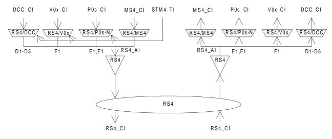
Figure 36: STM-4 Regenerator Section atomic functions
