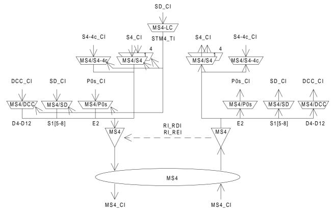
Figure 51: STM-4 Multiplex Section atomic functions
