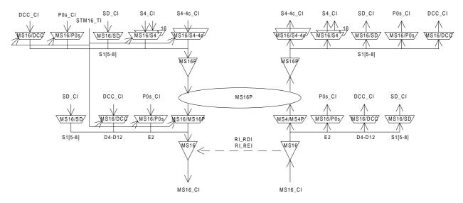
Figure 92: STM-16 Multiplex Section Linear Trail Protection Functions
