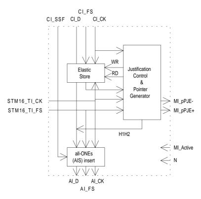
Figure 98: Main processes within MS16/S4\_A\_So
