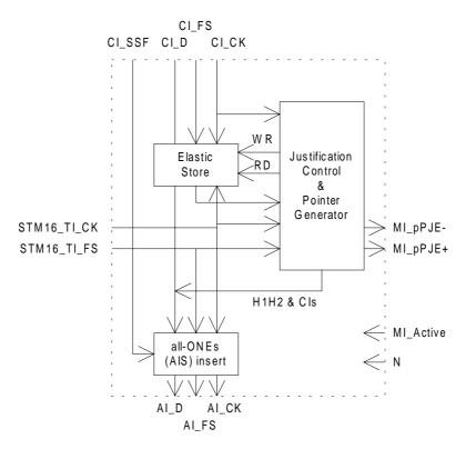
Figure 101: Main processes within MS16/S4-4c\_A\_So
