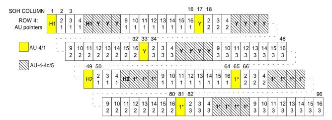
Figure C.5: AU pointers in STM-16 supporting AU examples in figure C.4 (in serial format)
