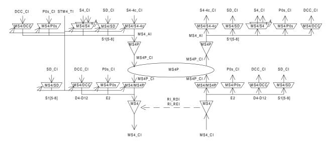
Figure 54: STM-4 Multiplex Section Linear Trail Protection Functions
