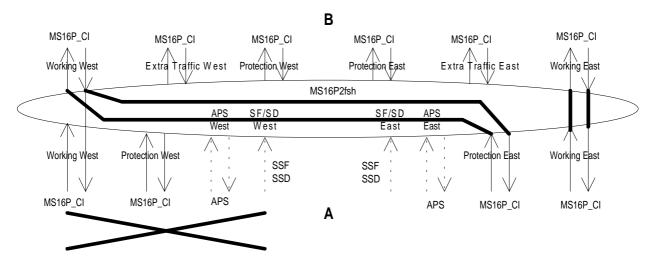
Figure 117: Matrix connections in a network element adjacent to a fault on its west side
