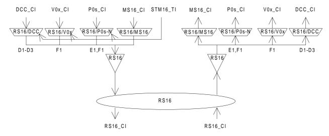
Figure 74: STM-16 Regenerator Section atomic functions
