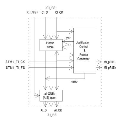
Figure 24: Main processes within MS1/S4\_A\_So
