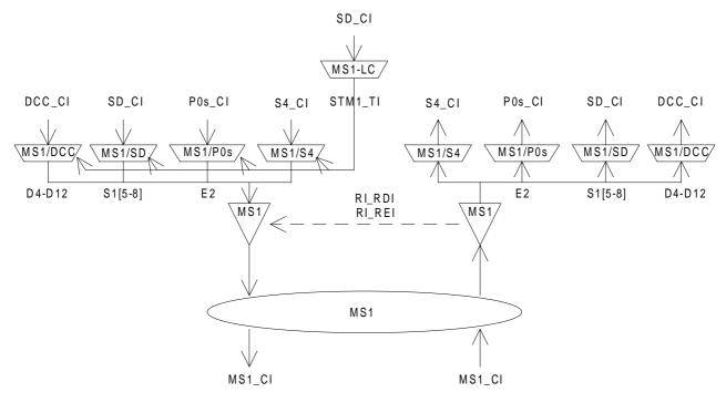
Figure 16: STM-1 Multiplex Section atomic functions
