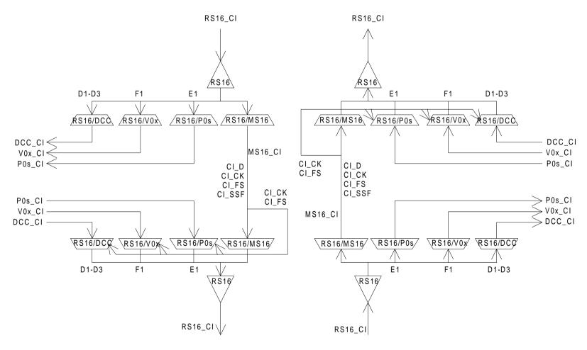
Figure B.1: STM-16 regenerator model (supporting DCC, OW, USR)
