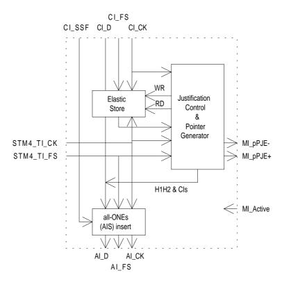
Figure 62: Main processes within MS4/S4-4c\_A\_So
