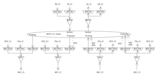
Figure D.1: 1+1 STM-1 Multiplex Section Linear Trail Protection model (unprotected DCC, OW, protected SSM)
