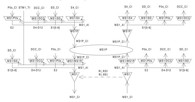
Figure 19: STM-1 Multiplex Section Linear Trail Protection Functions
