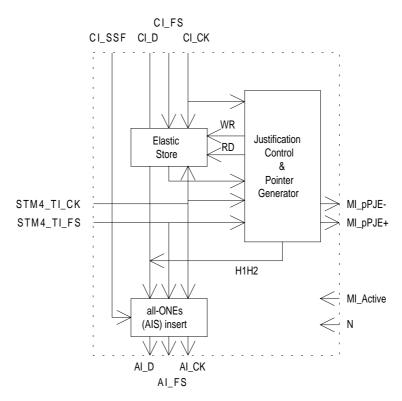
Figure 59: Main processes within MS4/S4\_A\_So
