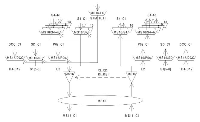
Figure 89: STM-16 Multiplex Section atomic functions
