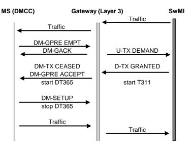
Figure 24: DM-MS pre-emption for continuation of ongoing call
