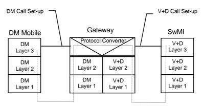
Figure 1: Protocol stack for gateway
