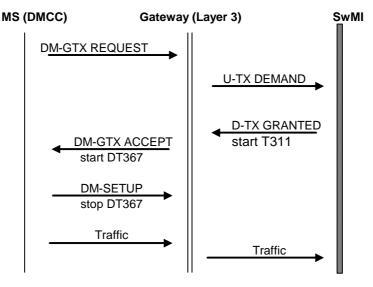
Figure 21: DM transmit request during DM channel reservation
