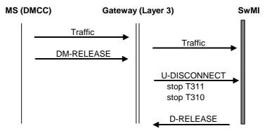
Figure 22: Call disconnection by master DM-MS
