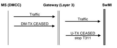
Figure 20: End of traffic transmission by master DM-MS
