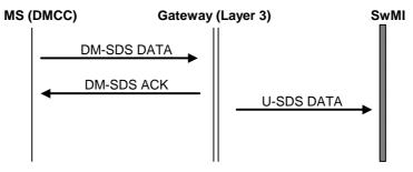
Figure 28: Outgoing DM SDS message to TMO
