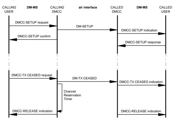
Figure 12: Call set-up without presence check
