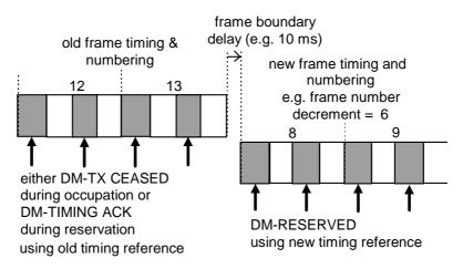
Figure 33: Timing adjustment illustration
