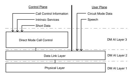
Figure 8: Protocol stack for MS functionality
