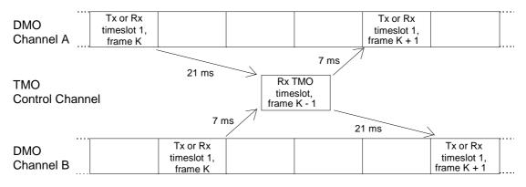
Figure 30: Full Dual watch timing on A and B channels
