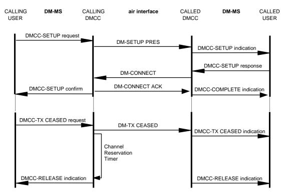
Figure 13: Call set-up with presence check
