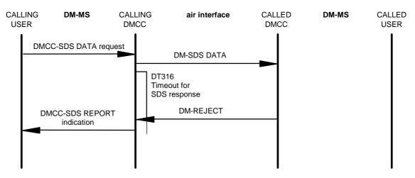
Figure 20: Acknowledged SDS message (rejected)
