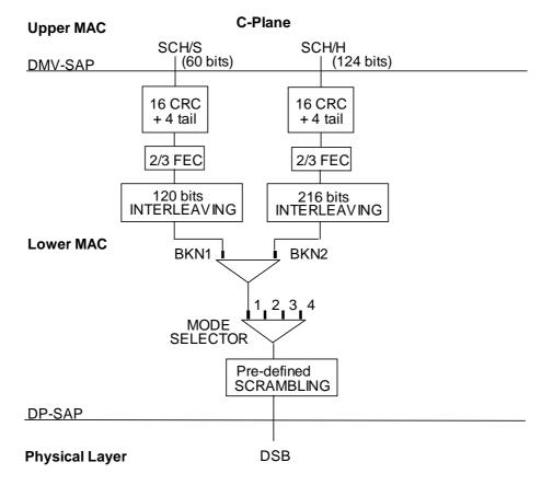
Figure 26: DM-MS configuration in sync signalling mode
