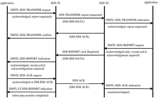
Figure 22H: SDS acknowledged transfer and report requested using acknowledged service, acknowledgement to report required
