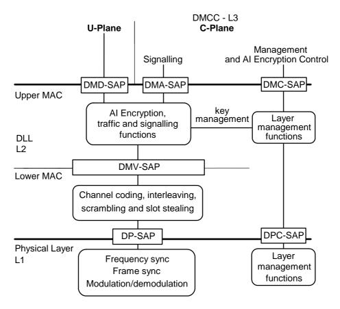
Figure 23: Layer 2 reference architecture
