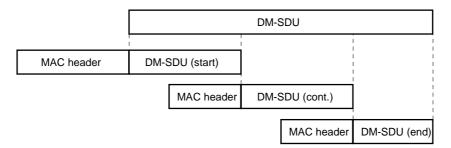
Figure 34: MAC fragmentation of a long DM-SDU
