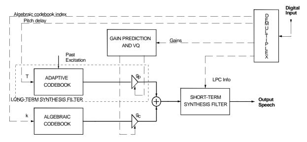
Figure 1: High level block diagram of the TETRA speech synthesizer
