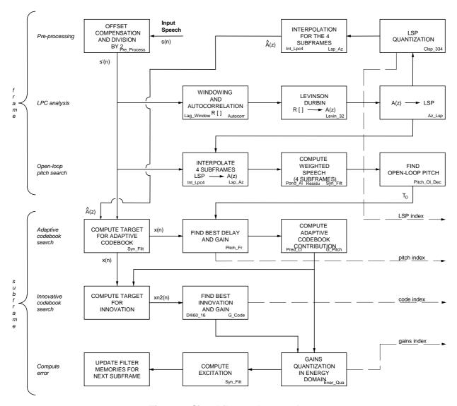
Figure 3: Signal flow at the encoder
