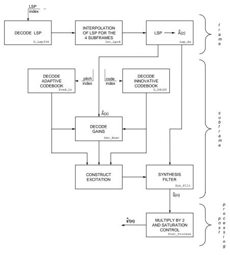
Figure 5: Signal flow at the decoder
