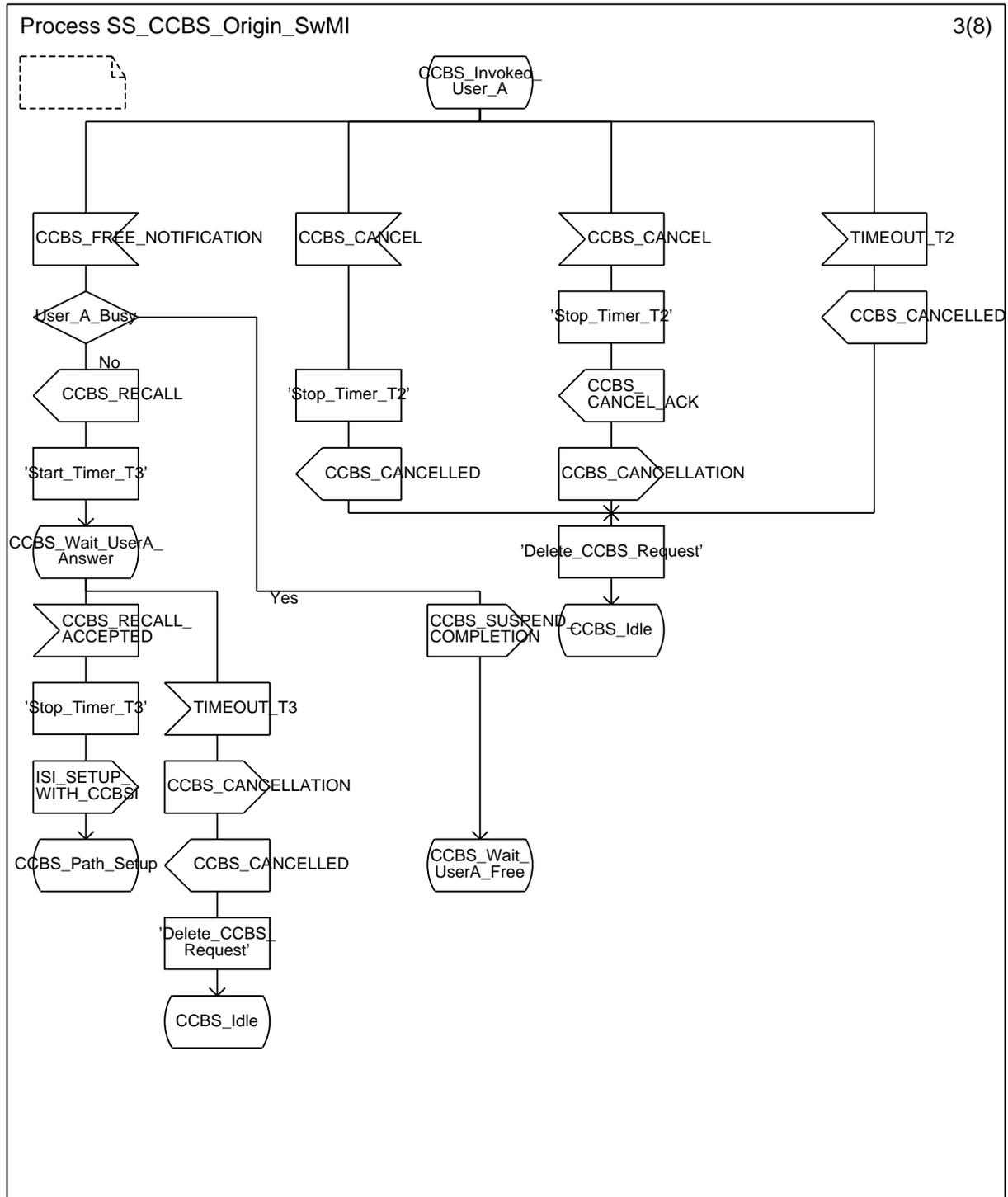
Figure A.1: Originating SwMI process (sheet 3 of 8)
