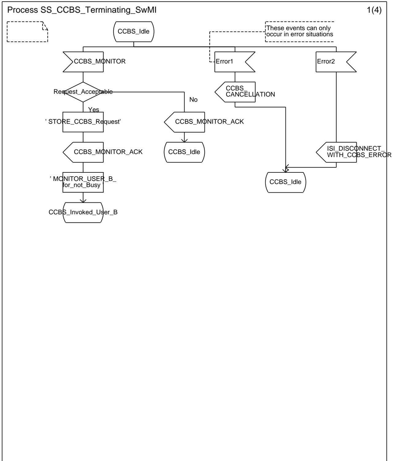
Figure A.2: Terminating SwMI process (sheet 1 of 4)
