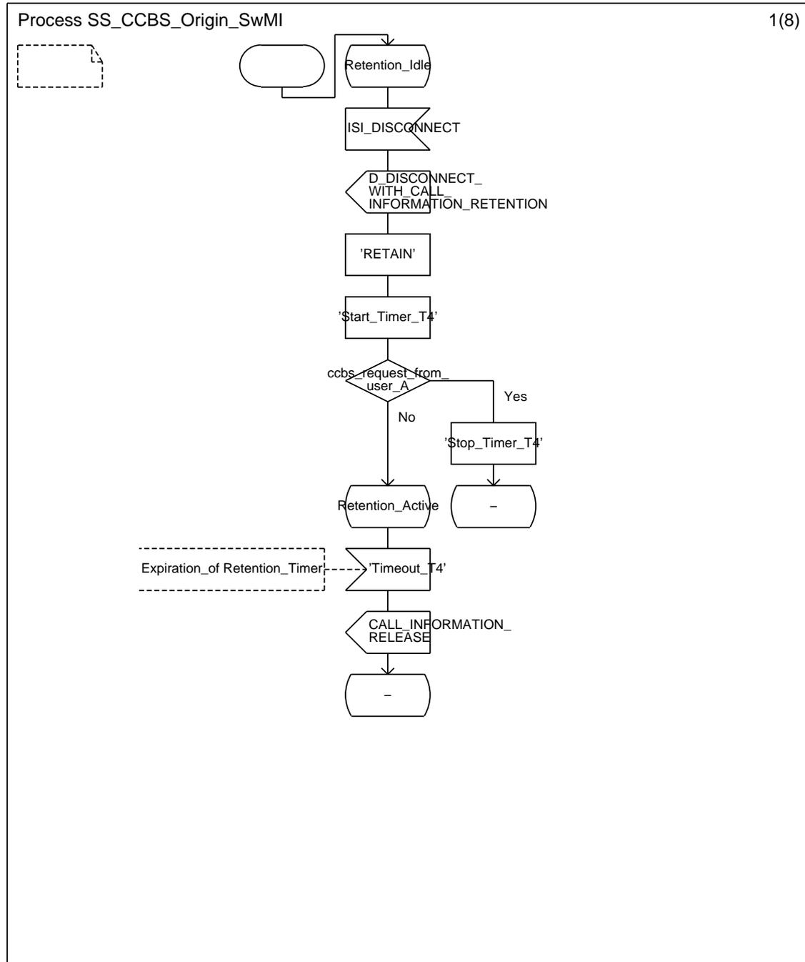
Figure A.1: Originating SwMI process (sheet 1 of 8)
