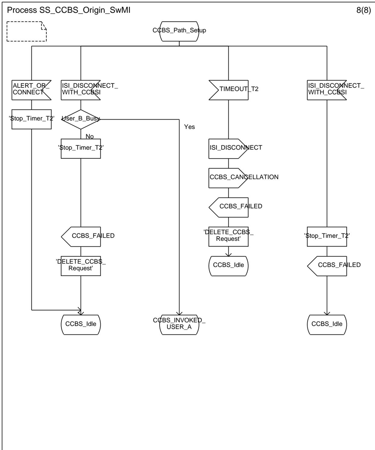
Figure A.1: Originating SwMI process (sheet 8 of 8)
