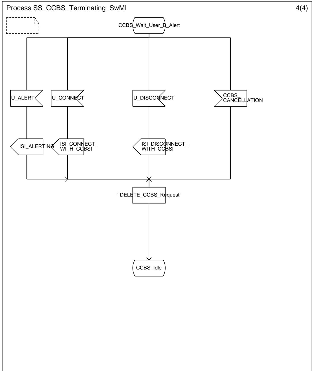
Figure A.2: Terminating SwMI process (sheet 4 of 4)
