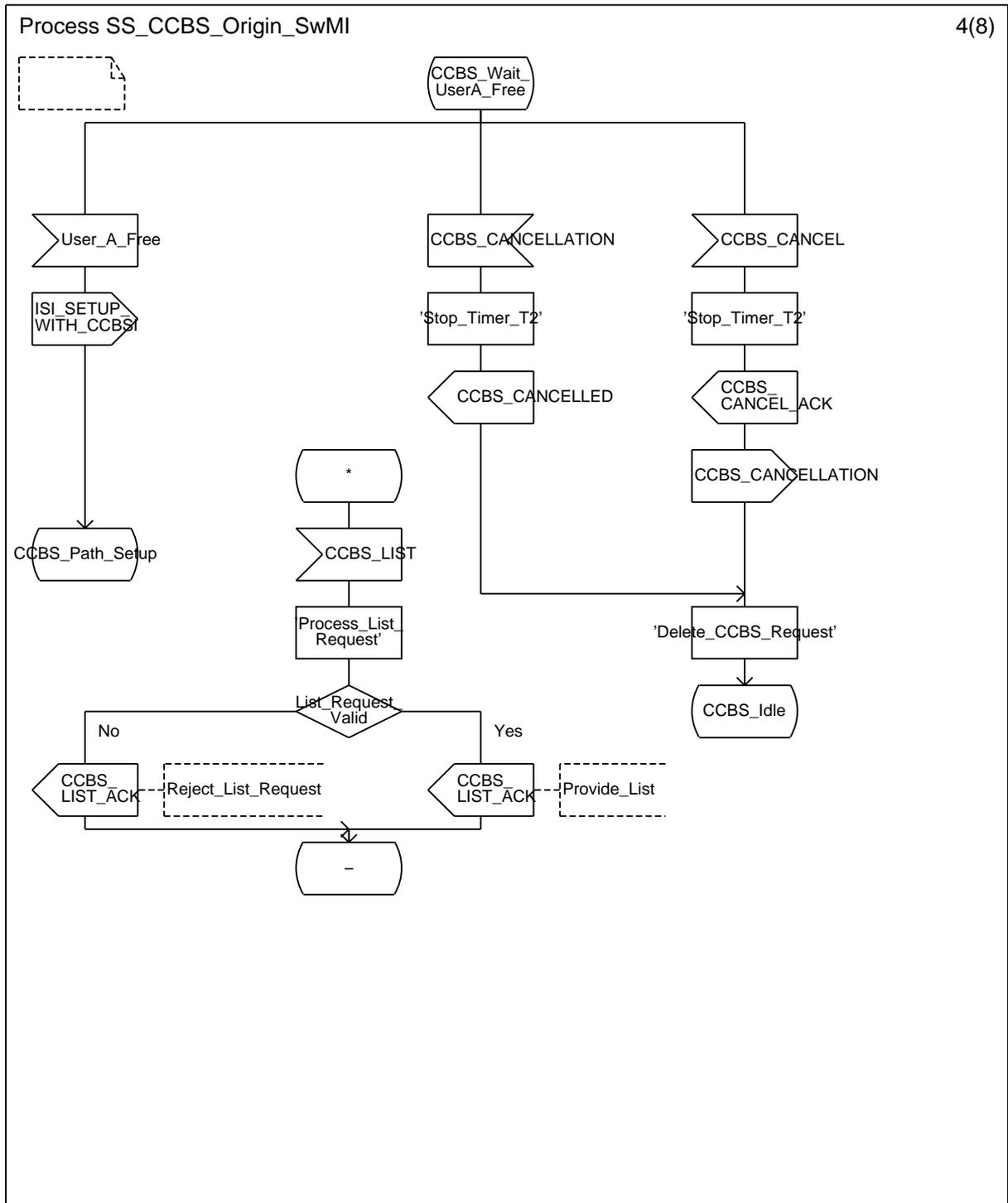
Figure A.1: Originating SwMI process (sheet 4 of 8)
