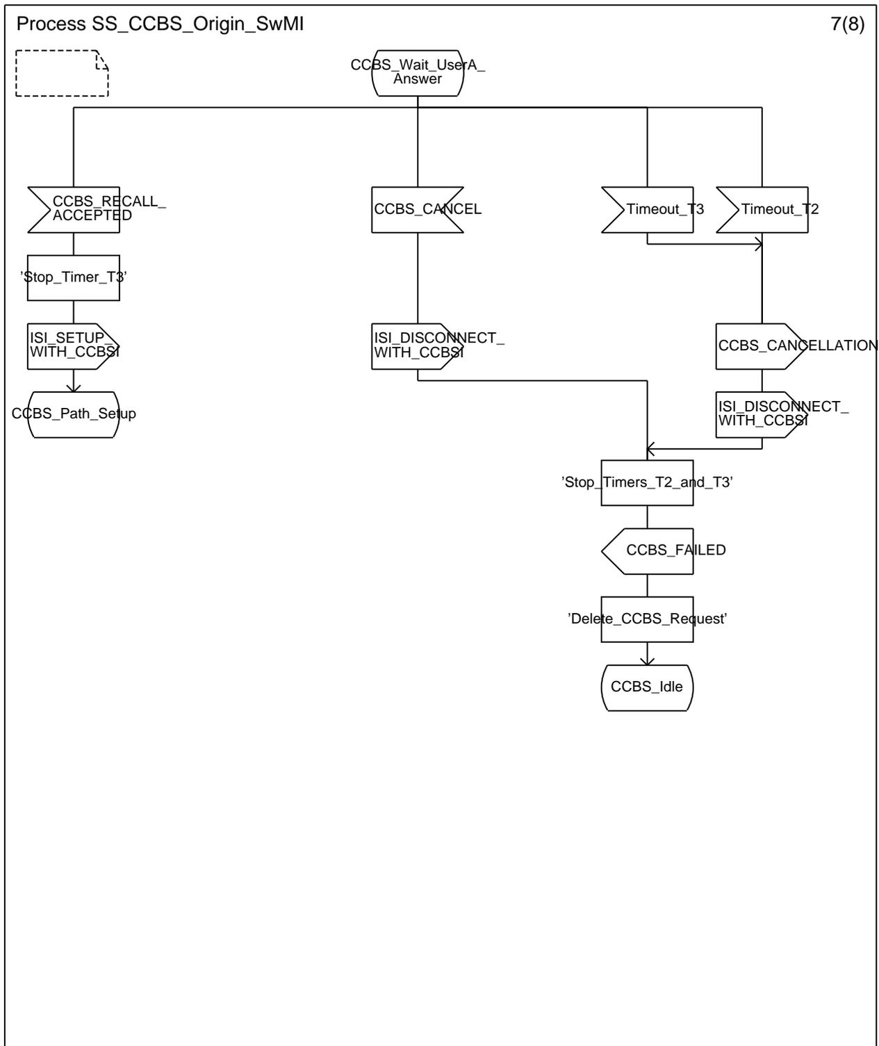
Figure A.1: Originating SwMI process (sheet 7 of 8)
