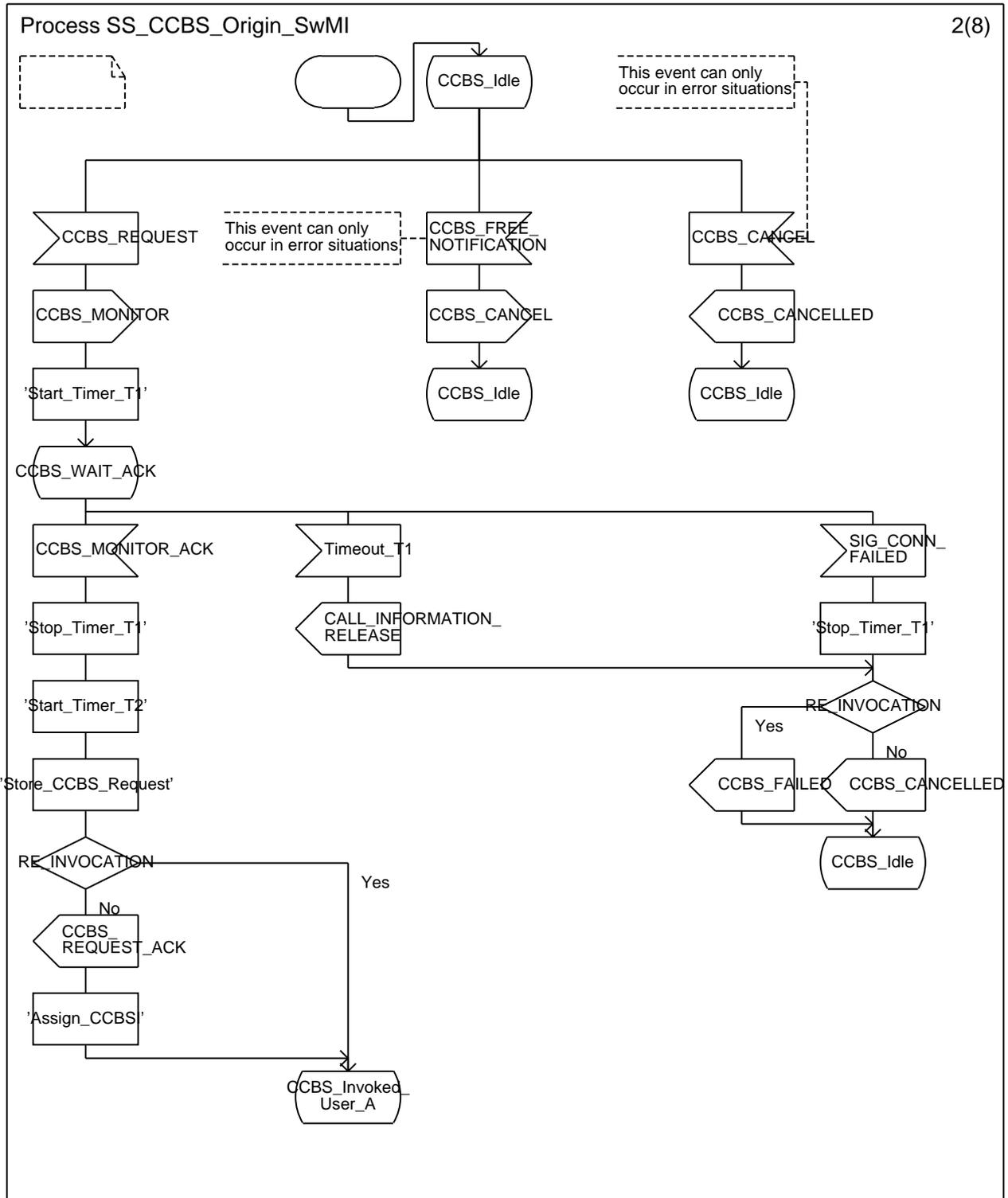
Figure A.1: Originating SwMI process (sheet 2 of 8)
