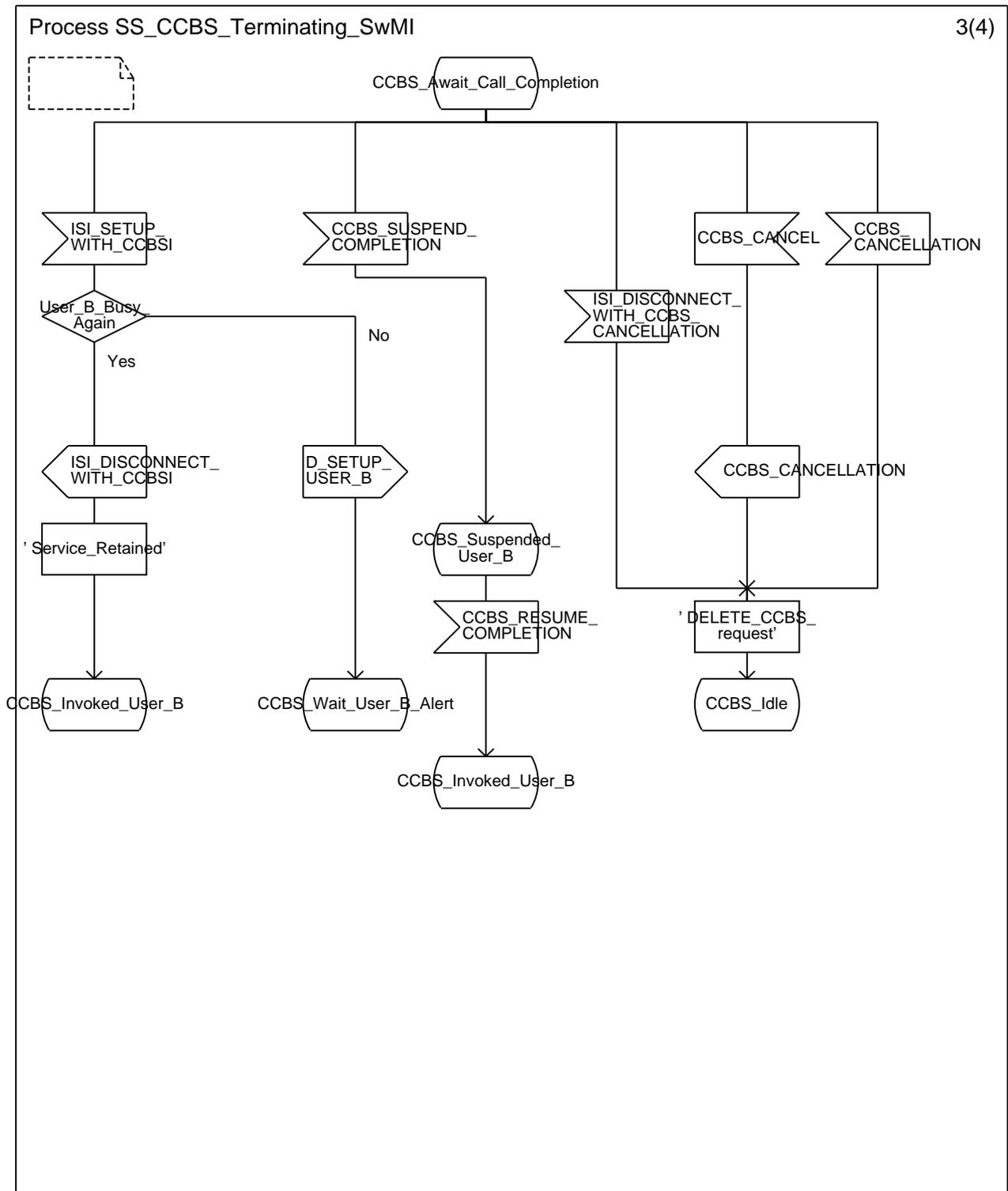
Figure A.2: Terminating SwMI process (sheet 3 of 4)
