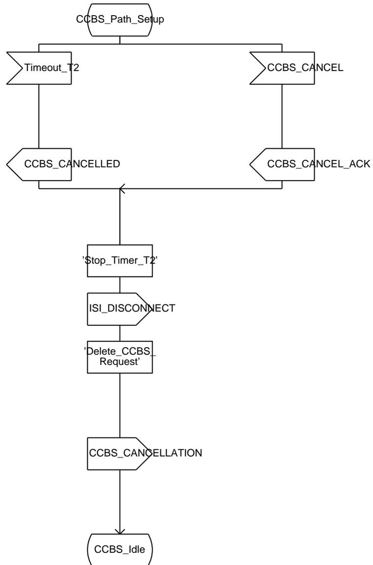
Figure A.1: Originating SwMI process (sheet 6 of 8)
