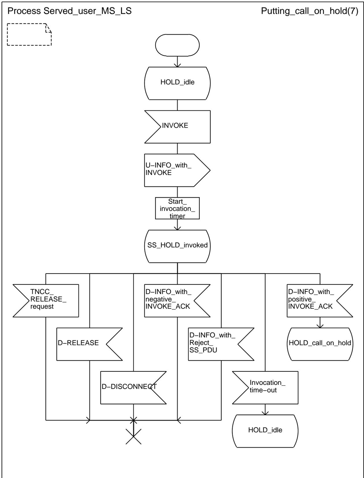
Figure B.1 (sheet 1 of 7): Served user MS/LS SDL - Invocation and beginning of operation
