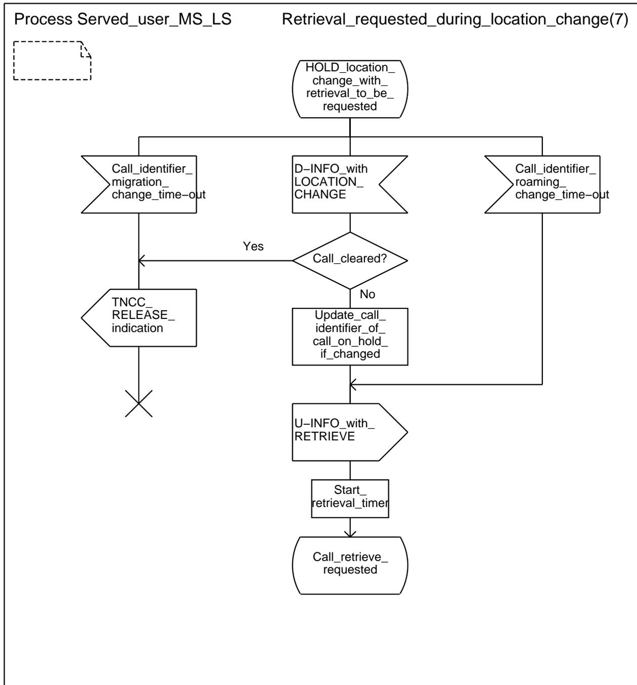
Figure B.1 (sheet 3 of 7): Served user MS/LS SDL - Retrieve primitive received during roaming or migration
