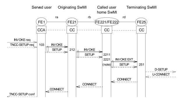
NOTE: In figures 8 and 9, since both FE21 and FE221 are collocated, in the originating SwMI, relationship rb will be internal to that SwMI.
