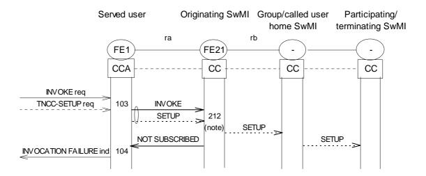
NOTE: The sequence shown in the figure shall always apply for all SS-AS invocations for individual calls (in the case of non-subscription). It shall only apply for SS-AS invocations for group calls when the originating SwMI has already been attached to the group (still in the case of non-subscription).
