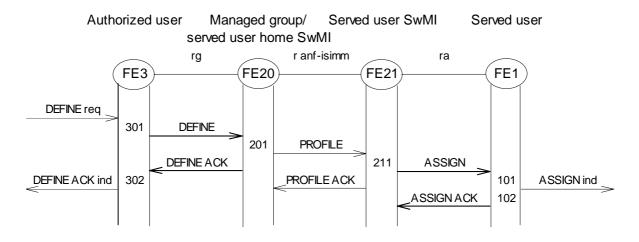
Figure 6: Definition of SS-AS with assignment to the served user(s)
