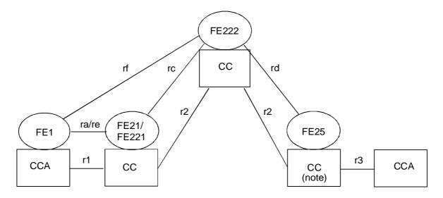
NOTE: The CC the called user CCA, on the right, is associated coincides with the transit CC shown in the middle of the figure (with FE222 collocated) when the called user is registered in his home SwMI (whether for an individual call or for a group call).
