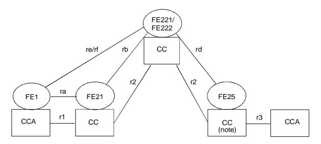
NOTE: The CC to which the called user CCA, on the right, is associated coincides with the transit CC shown in the middle of the figure (with FE221 and FE222 collocated) when the called user is registered in his home SwMI (whether for an individual call or for a group call).
