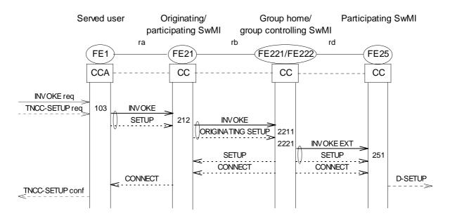
Figure 13: Basic invocation and operation of SS-AS over ISI - successful establishment of group call when the selected area definition is given in the group home SwMI and the originating SwMI lies wholly within the selected area
