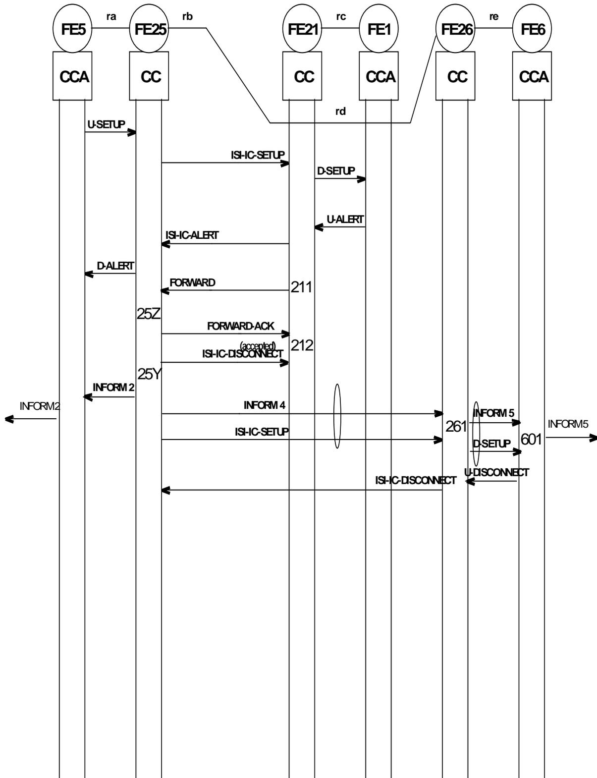
Figure 19: Information flow sequences for unsuccessful CFNRy operation: CFNRy not completed, original call cleared; case of re-routing
