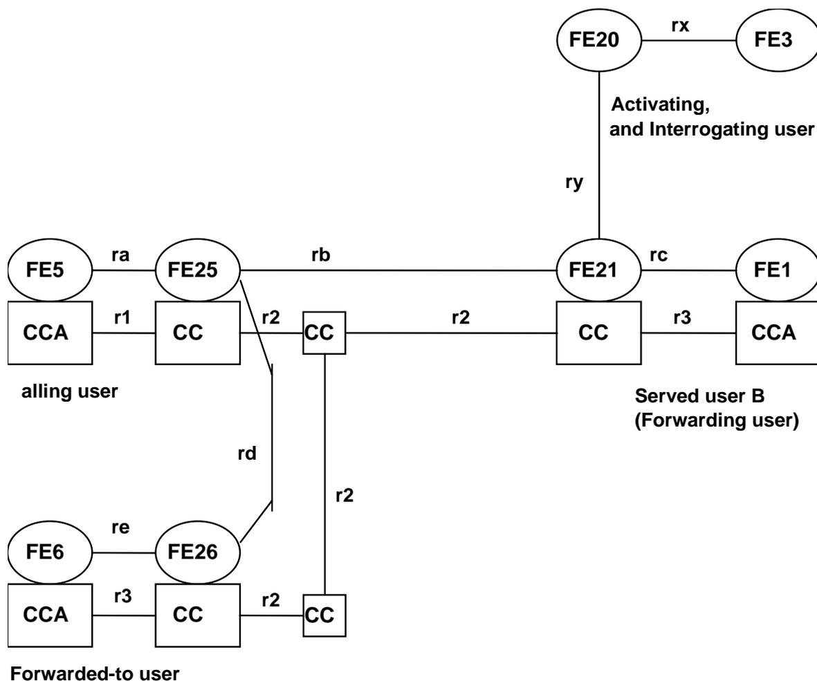
Figure 11: Functional Entity Model Relationship in Case of Individual Call, Single Stage Call Forwarding and Re-Routeing
