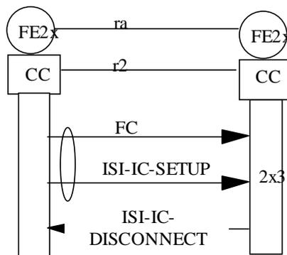
Figure 27: Information flow sequence; forwarding counter limit exceeded
