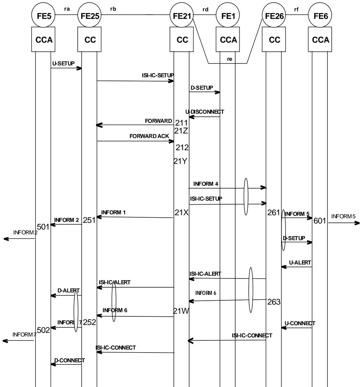
Figure 37: Information flow sequence for successful CFU/CFB operation; case of forward switching
