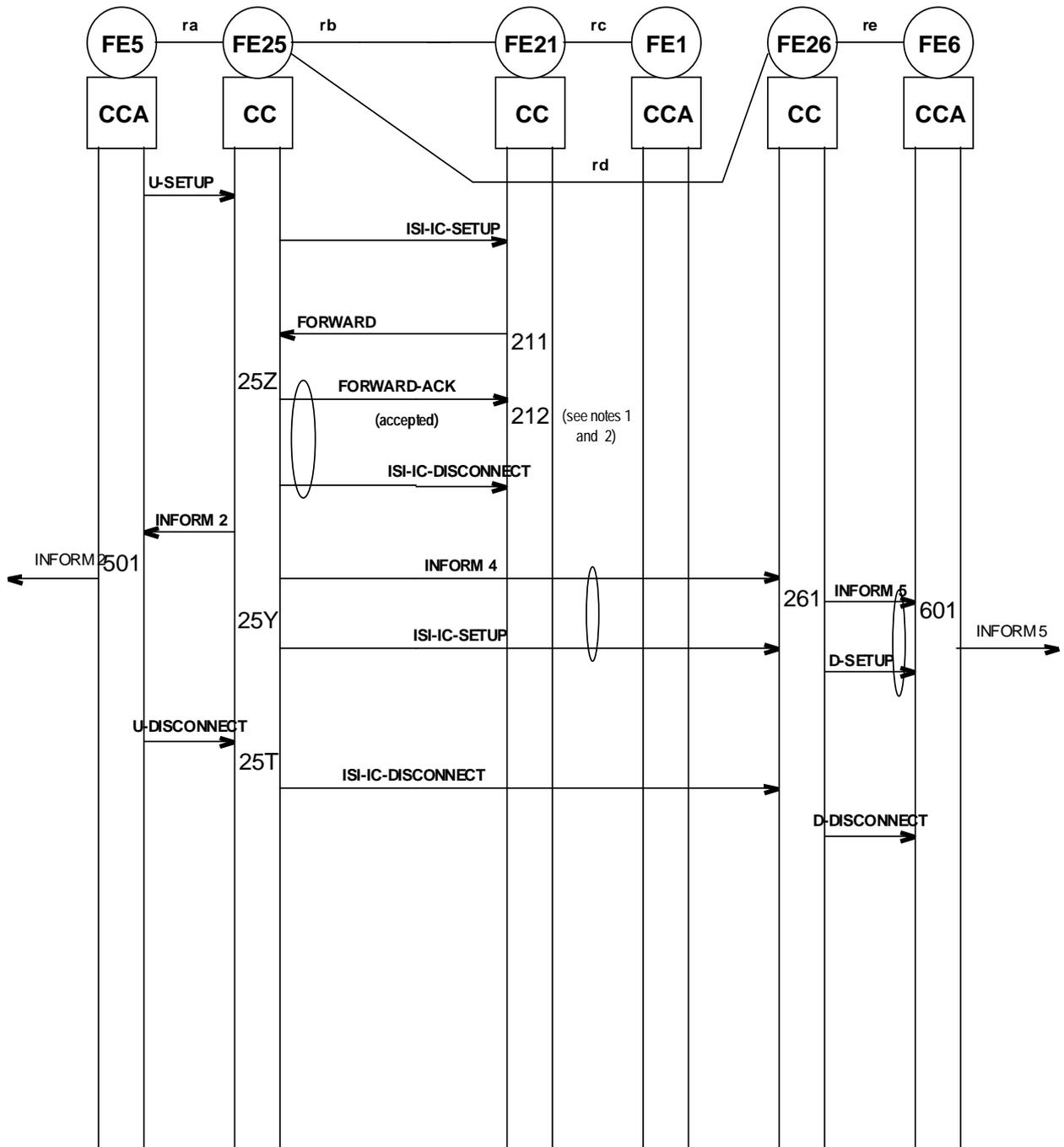
**Figure 22: Information flow sequence for clearing by user A during CFNRc operation; case of re-routing**
