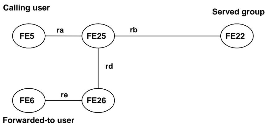
Figure 8: Functional entity model for group call, single stage of call forwarding (to an ITSI) and re-routing
