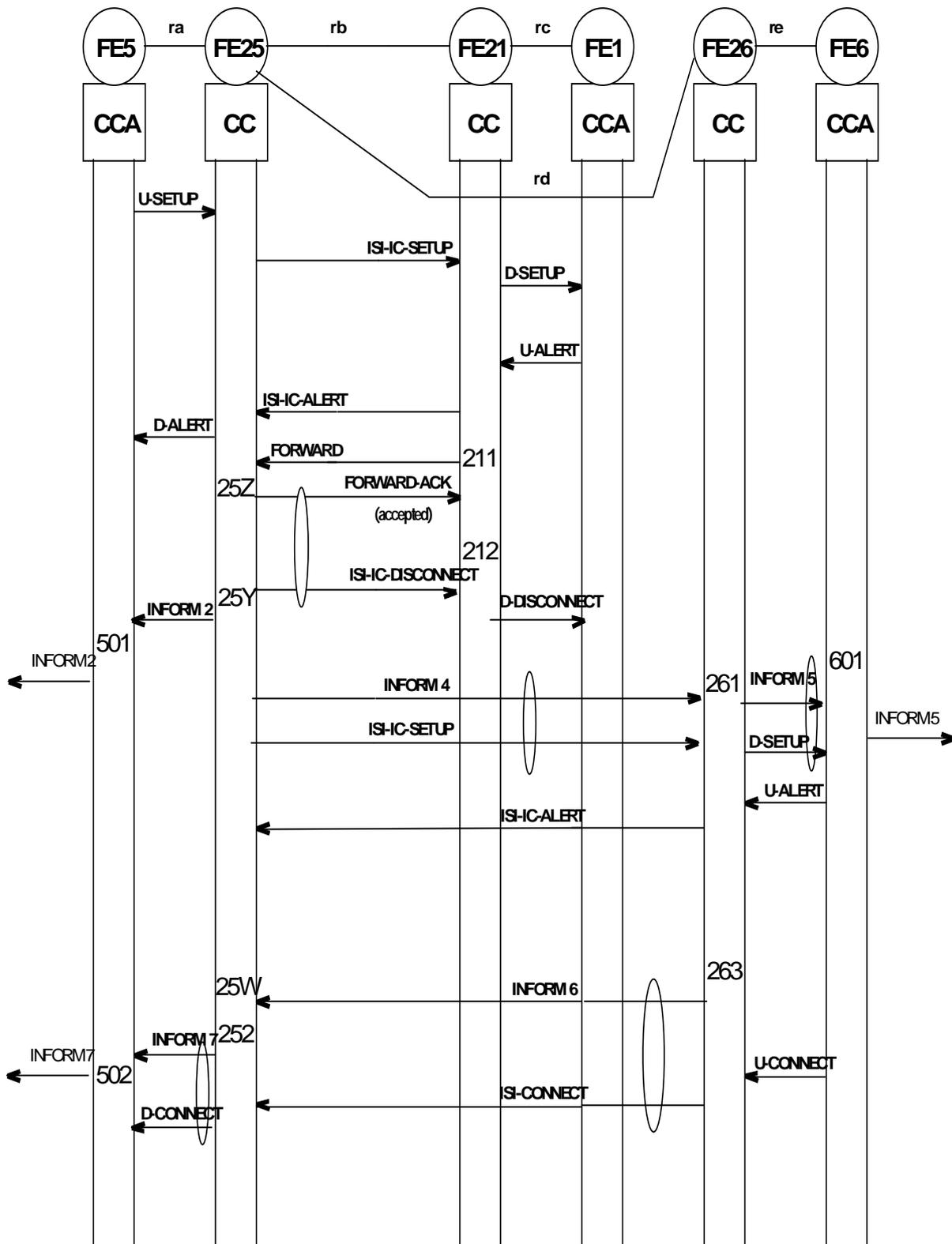
Figure 17: Information flow sequence for successful CFNRy operation; case of re-routeing
