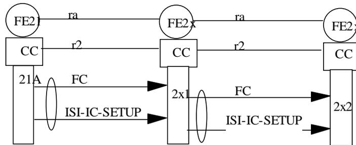
Figure 26: Information flow sequence; normal operation of FC
