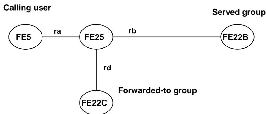
Figure 7: Functional entity model for group call, single stage of call forwarding and re-routing
