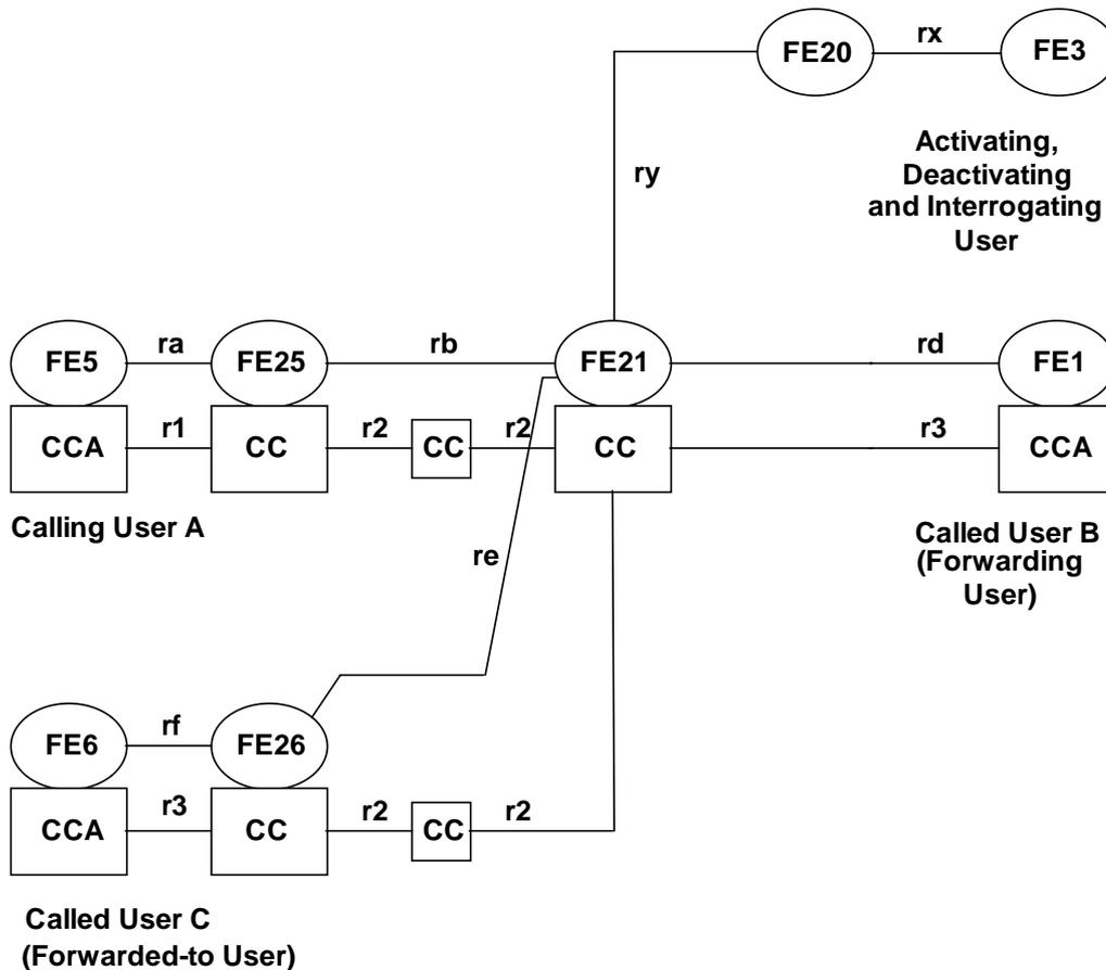
Figure 36: Functional entity model relationship, individual call, forward switching
