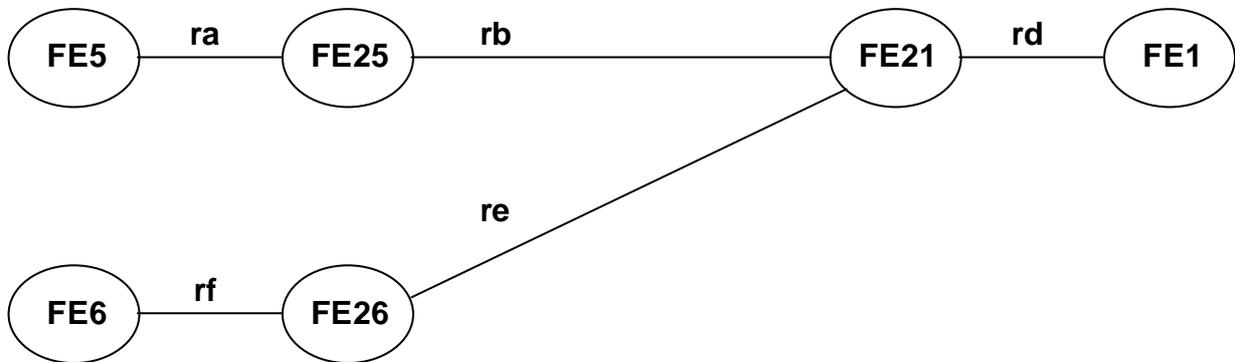
Figure 34: Functional entity model for individual call, single stage of Call Forwarding and forward switching
