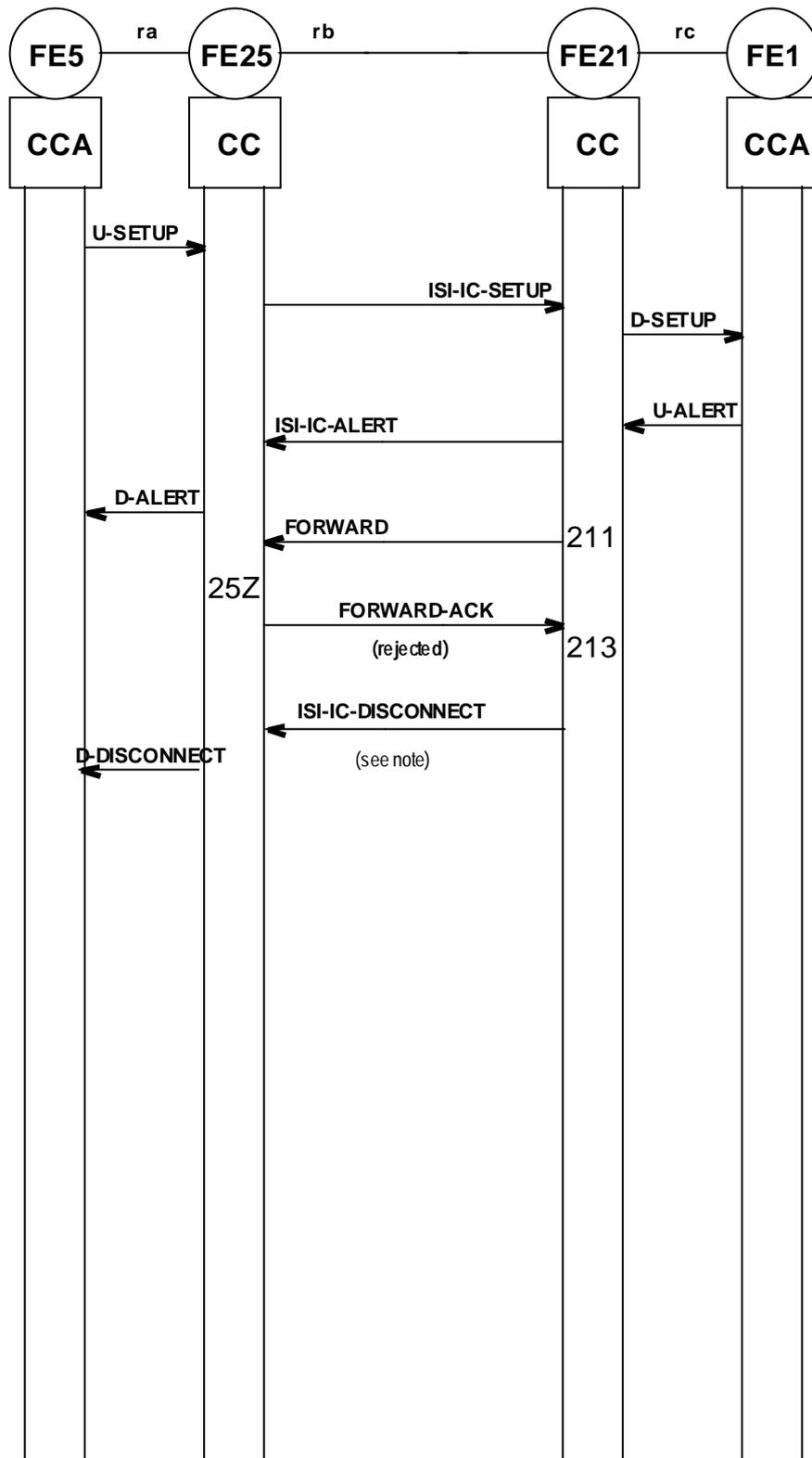
NOTE: With a disconnect cause "SS-specific disconnection".
