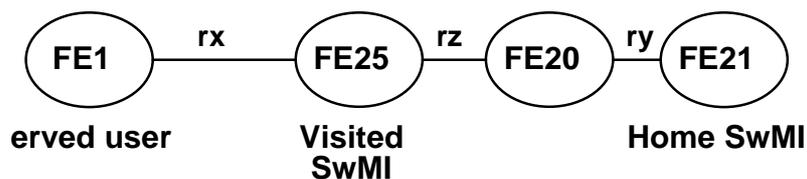
NOTE 1: In the case of local call forwarding, FE20 is collocated with FE21 and route ry is internal to FE21.
