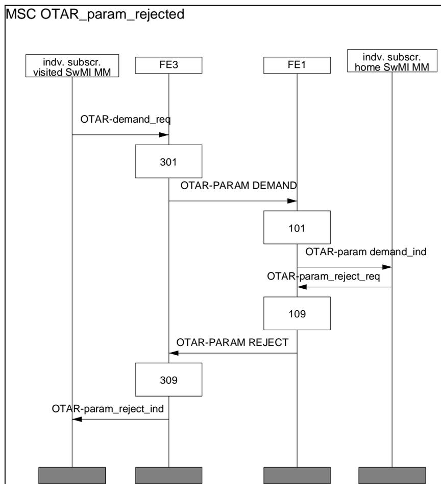
Figure 29.5: Failed OTAR parameter delivery
