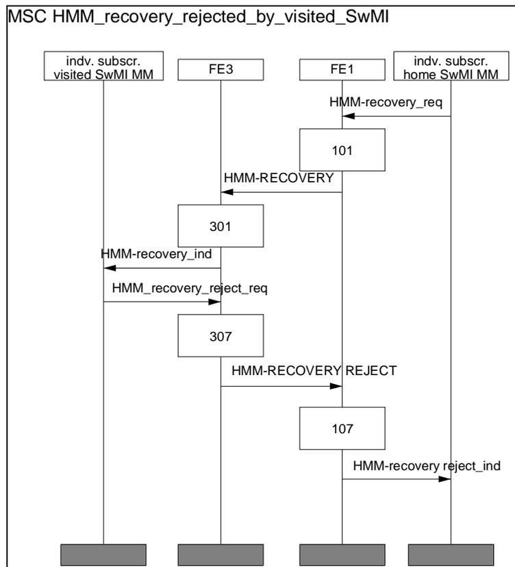
Figure 30.7: Rejection of HMM recovery
