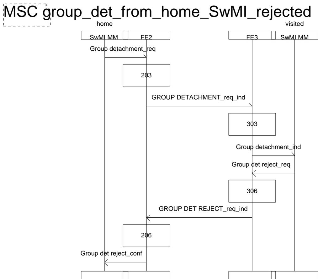
Figure 93: Rejection of group home SwMI MM initiated group detachment rejection
