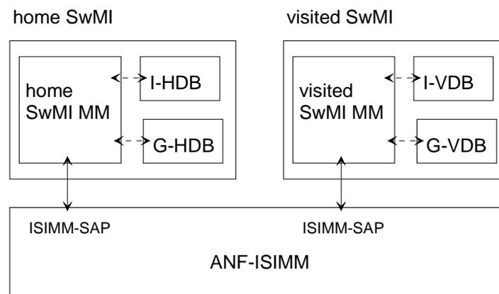
NOTE: The arrows illustrate the information exchange routes of the service. In the case of a solid arrow, the information exchange is mandatory; in the case of a broken arrow, the information exchange is conditional. If the service is invoked against an individual subscriber the I-HDB and the I-VDB are involved; if against group the G-HDB and the G-VDB are involved.
