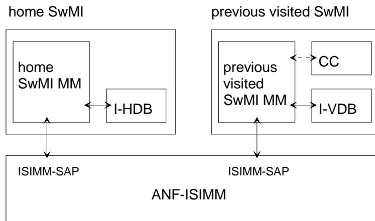
NOTE: The arrows illustrate the information exchange routes of the service. In the case of a solid arrow the information exchange is mandatory; in the case of a broken arrow the information exchange is conditional. The CC exists in the previous visited SwMI if the individual subscriber is engaged in a call when he migrates.
