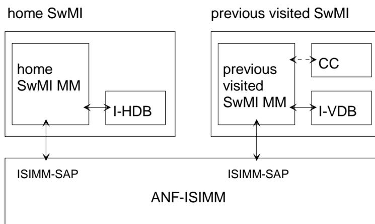
NOTE: The arrows illustrate the information exchange routes of the service. In the case of a solid arrow the information exchange is mandatory; in the case of a broken arrow the information exchange is conditional. The CC exists in the previous visited SwMI if the individual subscriber is engaged in a call when he migrates.
