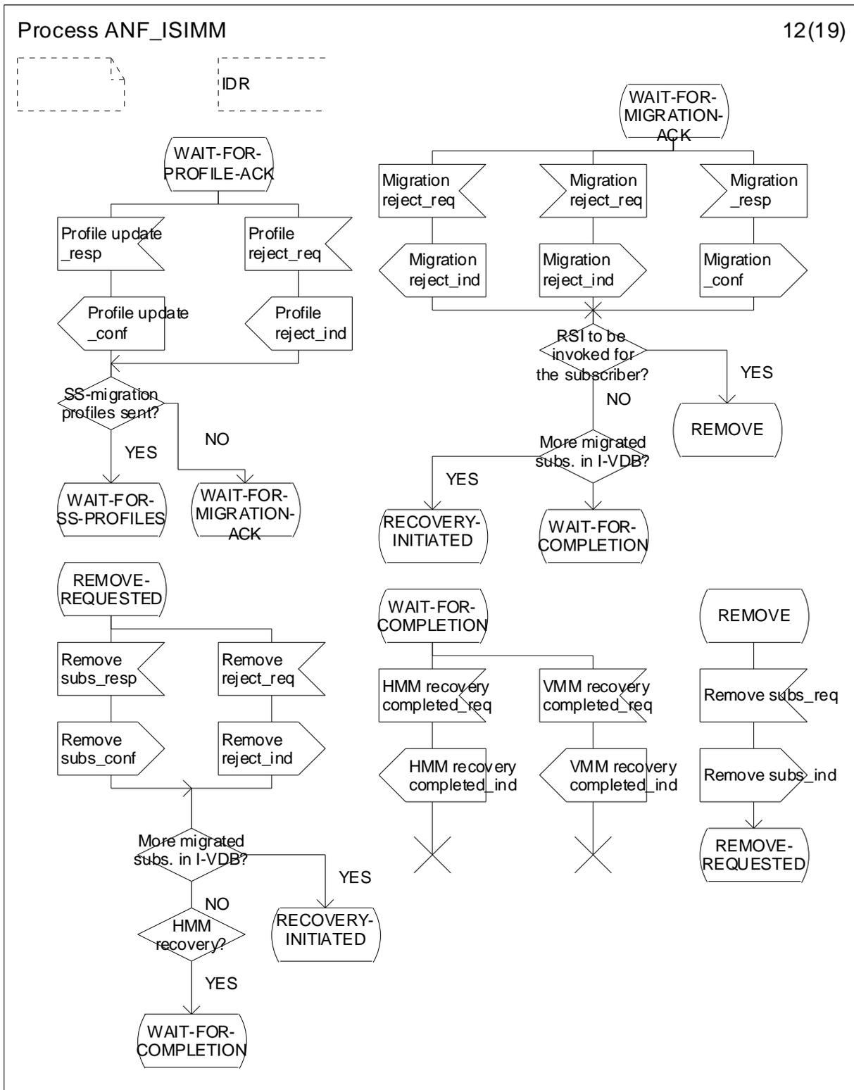
Figure 23: Stage 1 SDL description of IDR service
