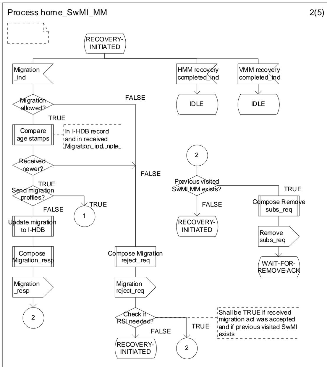
NOTE: If the received Migration\_ind is part of the HMM recovery, it is possible that there is no I-HDB record for the individual subscriber. If there is no I-HDB record for the subscriber the received Migration\_ind shall be considered as newer (i.e. shall not be rejected due to age stamp).
