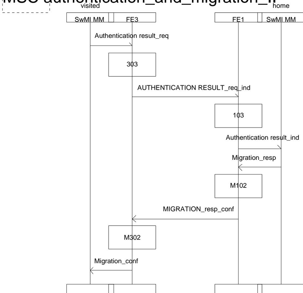
Figure 60: Authentication invoked in conjunction with migration (sheet 2 of 2)
