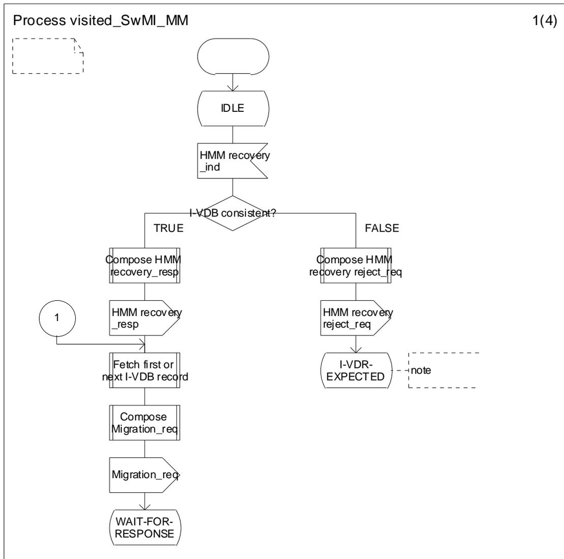
NOTE: If a SwMI MM rejects the recovery because its database is not able to support the recovery (it is not consistent) that SwMI MM shall invoke the recovery in order to recover the database.
