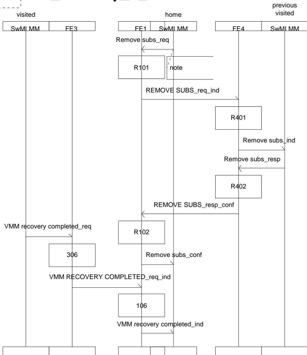
Figure 76: VMM recovery (sheet 3 of 3)
