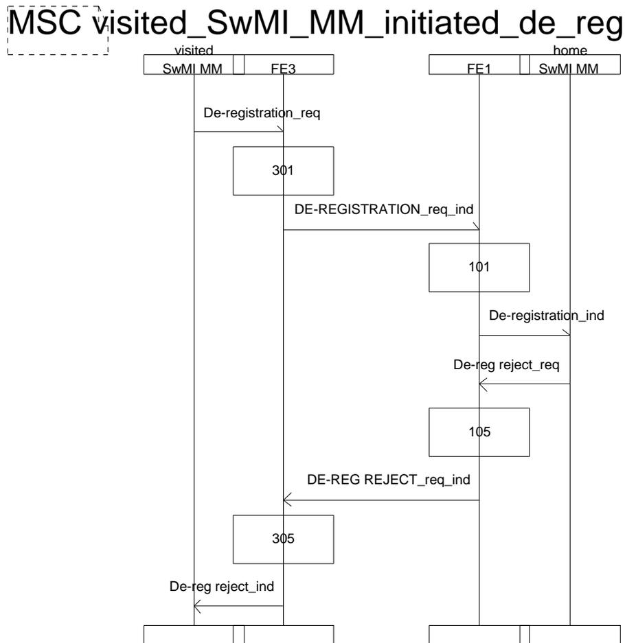
Figure 51: Visited SwMI MM initiated de-registration rejected
