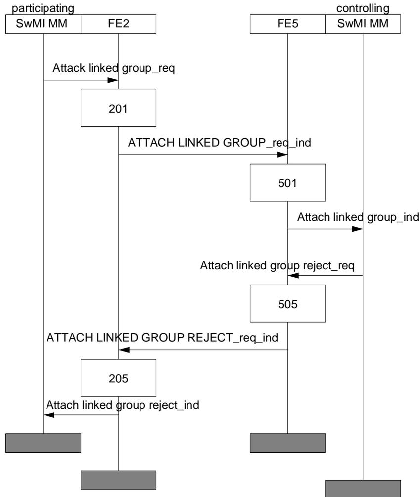
**Figure 107c: Visited SwMI MM initiated first group attachment to a linked group in the linking participating SwMI, rejected by the linking controlling SwMI**
