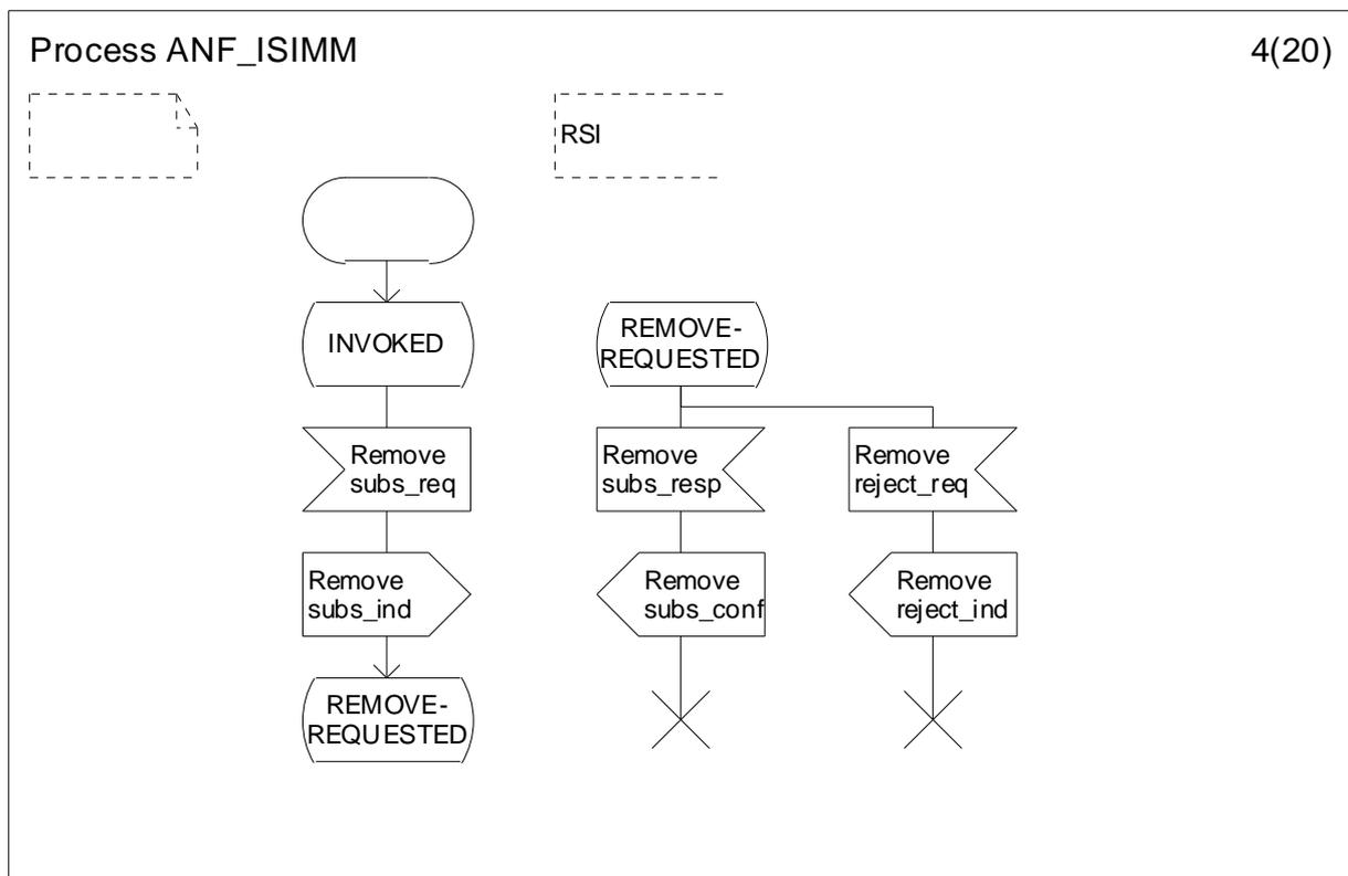
Figure 9: Dynamic description of RSI service using SDL
