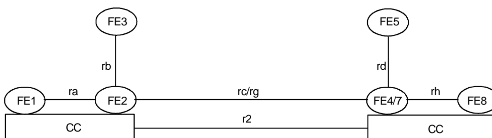
Figure 5: Example relationship between models for ANF-ISIIC and basic call in the case of called user hSwMI being SwMI B, with no migration
