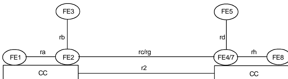
Figure 5: Example relationship between models for ANF-ISIIC and basic call in the case of called user hSwMI being SwMI B, with no migration
