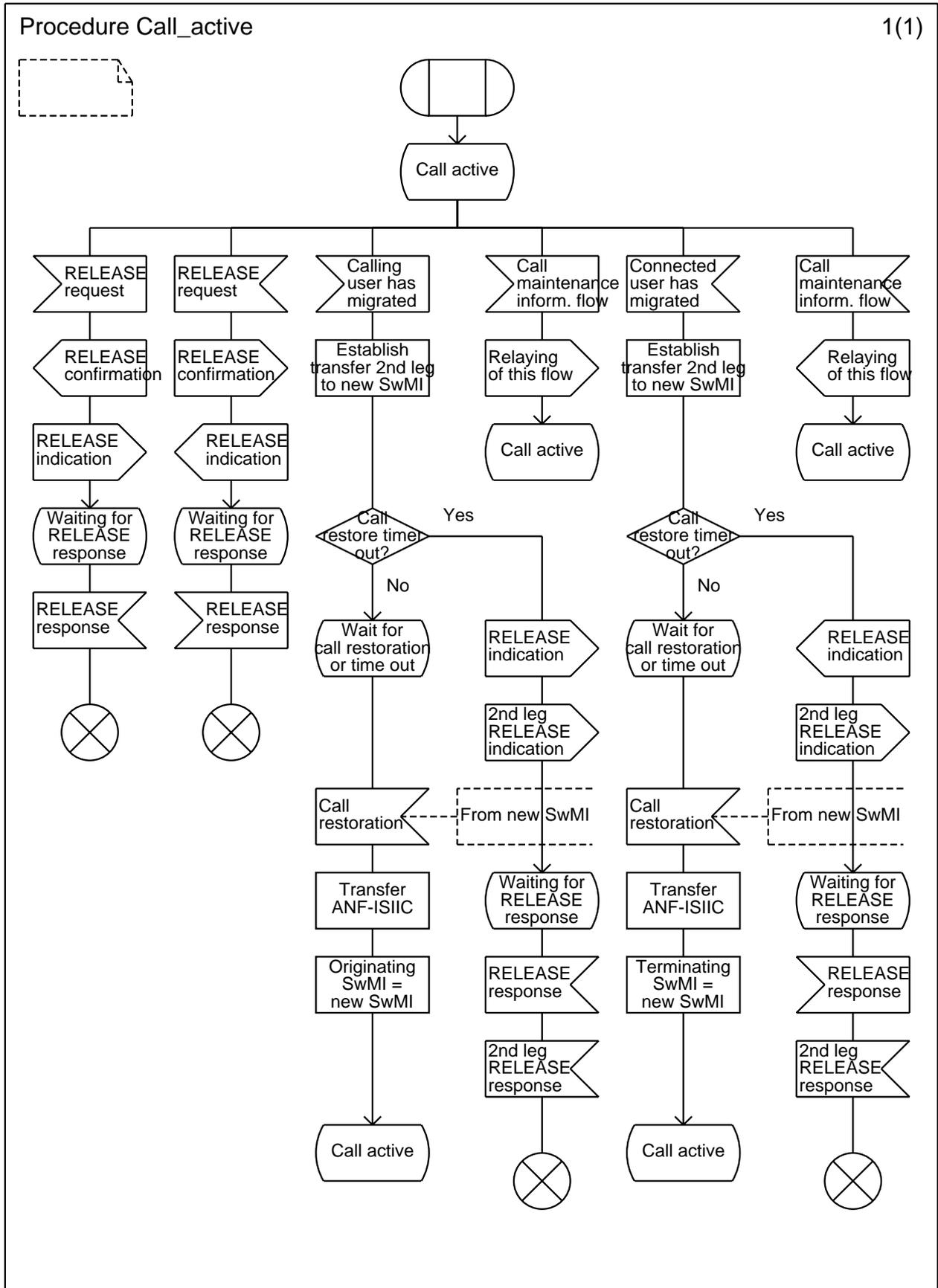
Figure 2 (sheet 4 of 5): ANF-ISIIC, overall SDL
