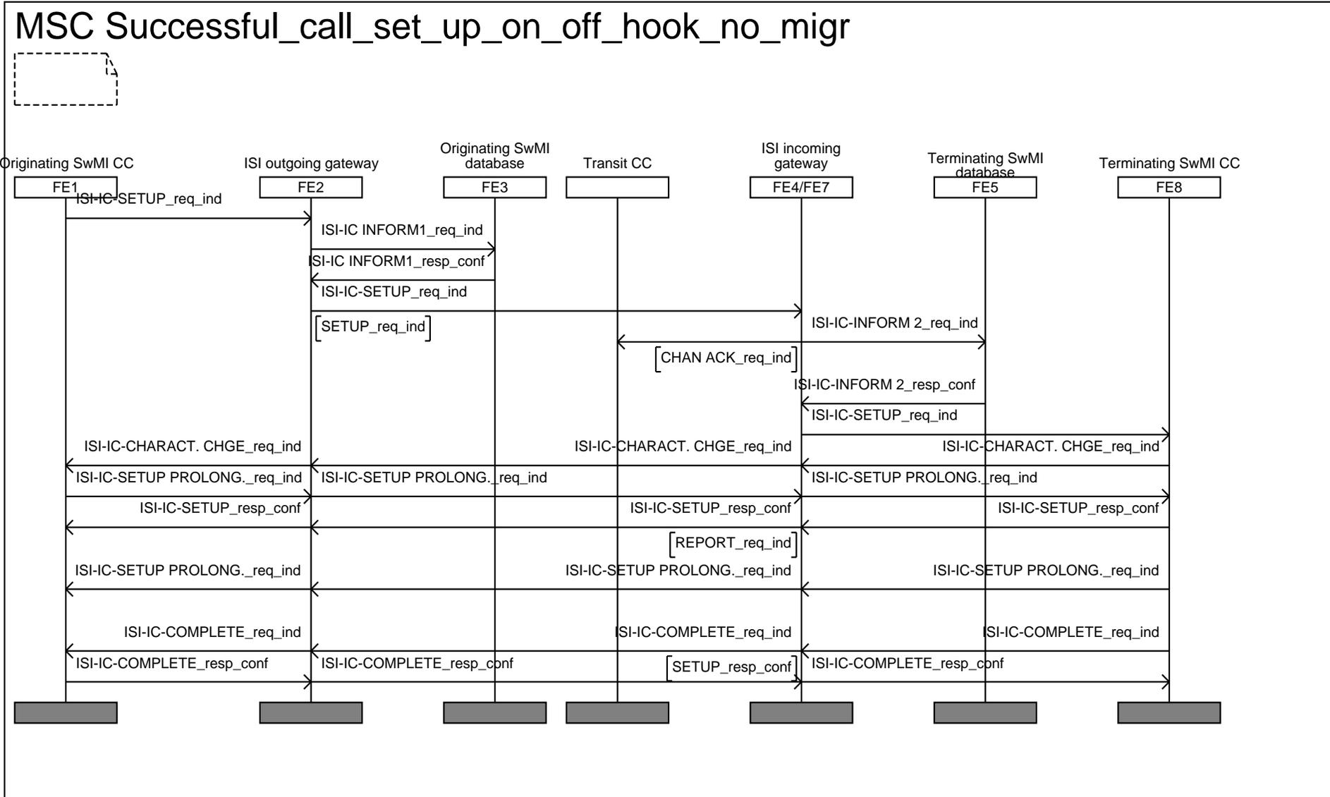
NOTE: The ISI-IC-SETUP PROLONGATION and -CHARACTERISTIC CHANGE request/indication information flows shown on the figure are optional.
