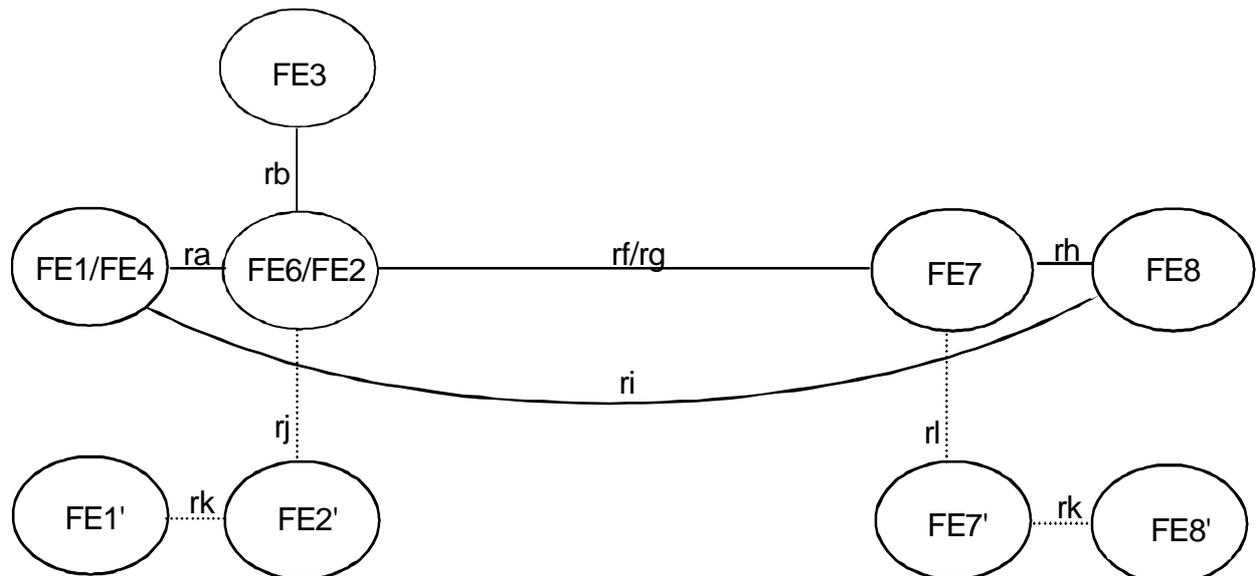
NOTE: Even though it is not a functional entity of ANF-ISIIC in this case (see subclause 5.1.2.4), FE4 has been shown in figure 4 to avoid showing a direct relationship between FE1 and FE6.
