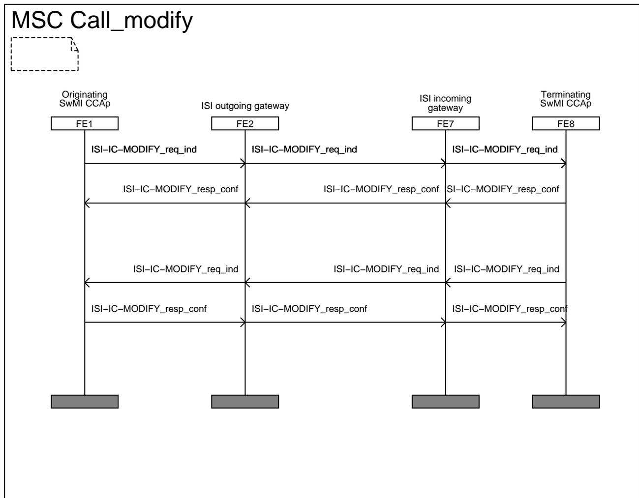
**NOTE:** The MODIFY information flows are not end-to-end between the originating and the terminating SwMI because they may result in a change in the 8 kbit/s encoding of the user information at the ISI, i.e. if the circuit mode service is modified, i.e. from speech to data service or vice-versa, or if the circuit mode service being data service, this service is changed, e.g. from 7,2 kbit/s to 4,8 kbit/s.
