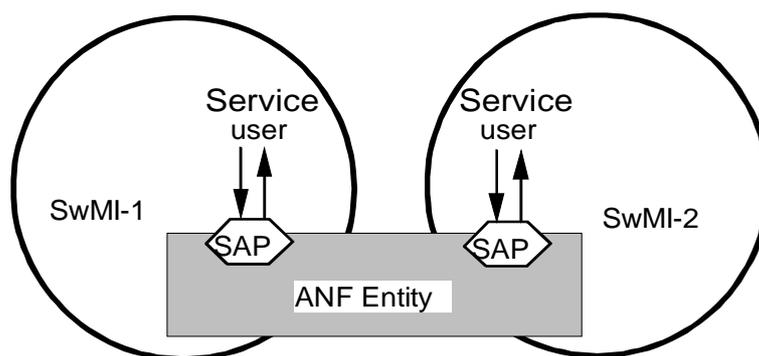
**Figure 1: Service model for point to point services**
