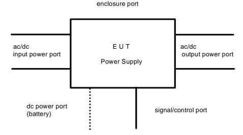
Figure 6: Port identifications of the EUT
