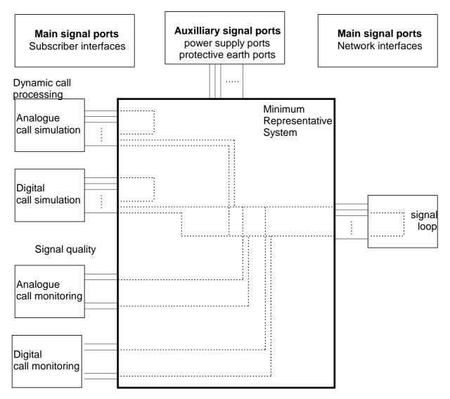
Figure 2: Schematic test configuration, switching equipment
