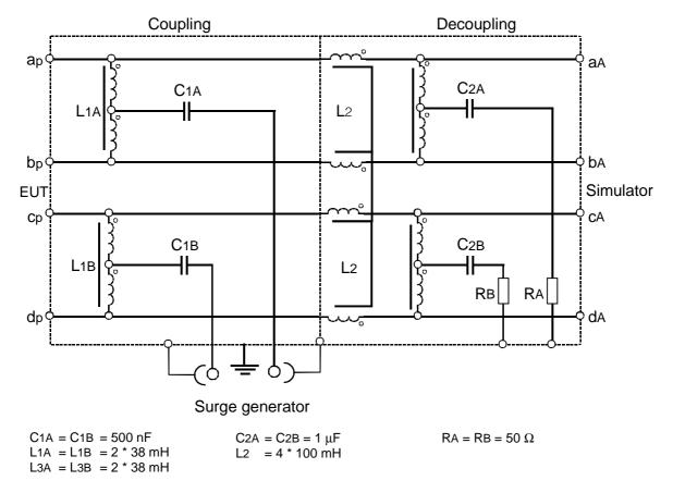
NOTE: L2 shall be a 4-coil current compensated choke to avoid saturation of coils due to phantom power feeding.
