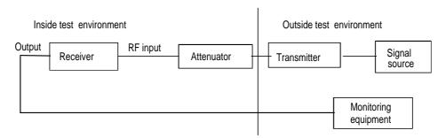
Figure 5: Test configuration for receivers
