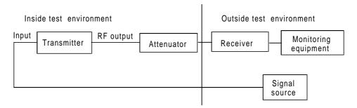
Figure 4: Test configuration for transmitters
