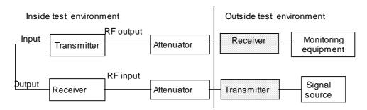
Figure 6: Test configuration of transceivers
