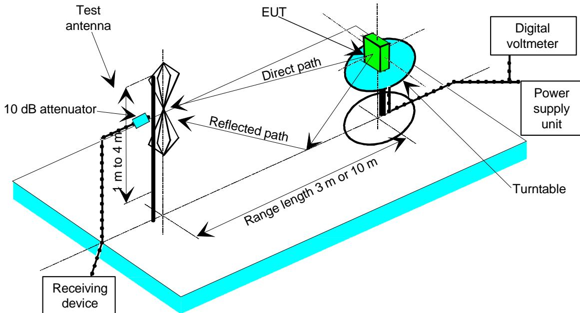
**Figure A.4: Measuring arrangement on ground plane test site
