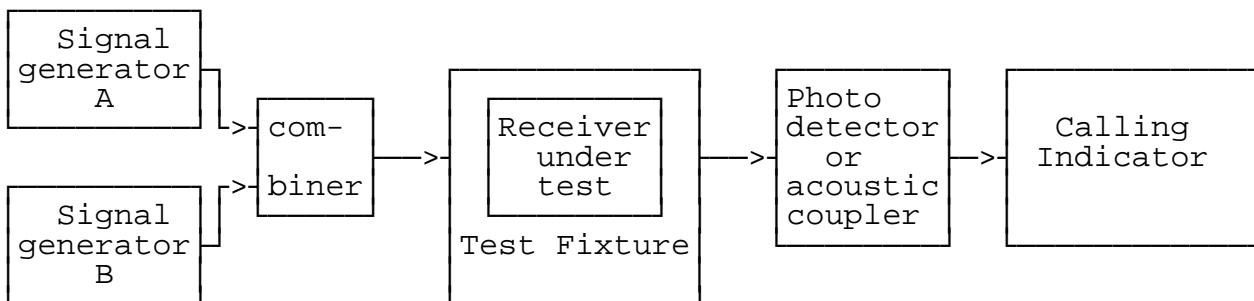
**Figure 13: Measurement arrangement**
