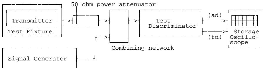
**Figure 8: Measurement arrangement**
