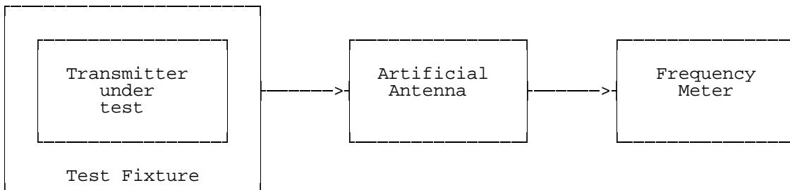
**Figure 1: Measurement arrangement**
