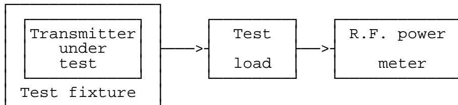
**Figure 4: Measurement arrangement**
