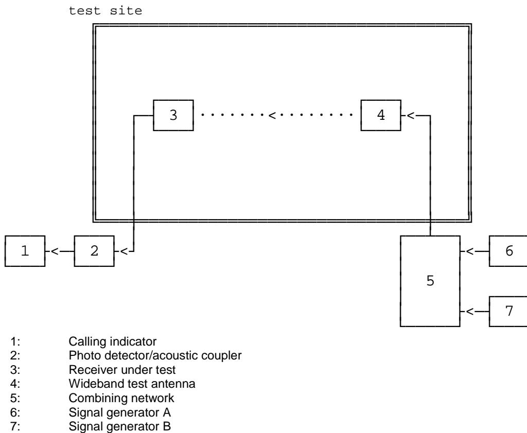
**Figure 16: Measurement arrangement**
