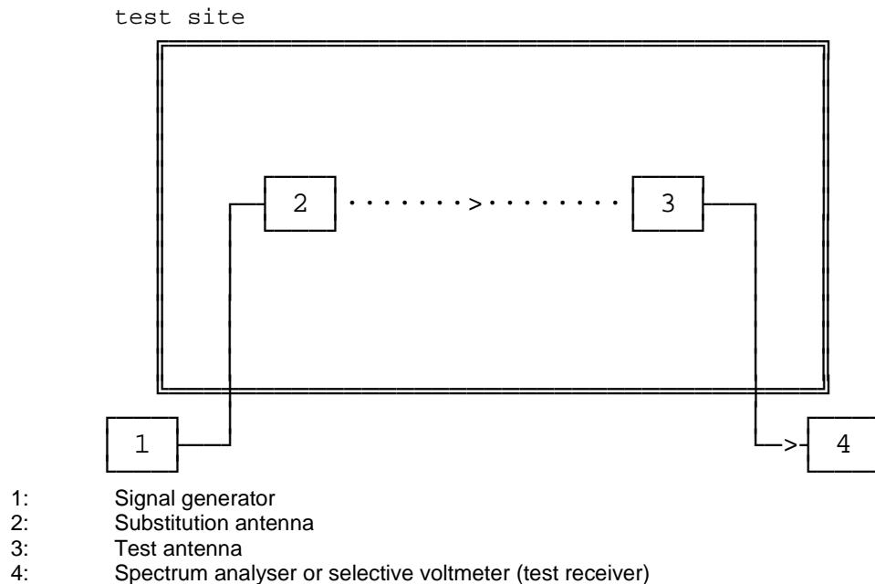
**Figure 18: Measurement arrangement**
