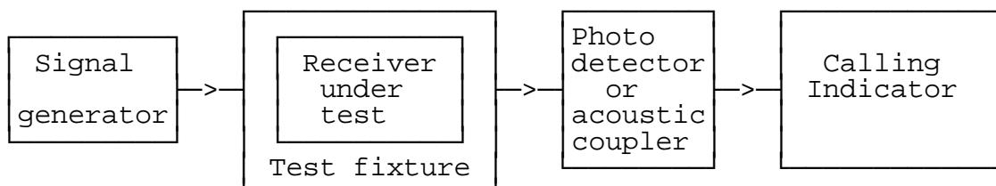
**Figure 11: Measurement arrangement**
