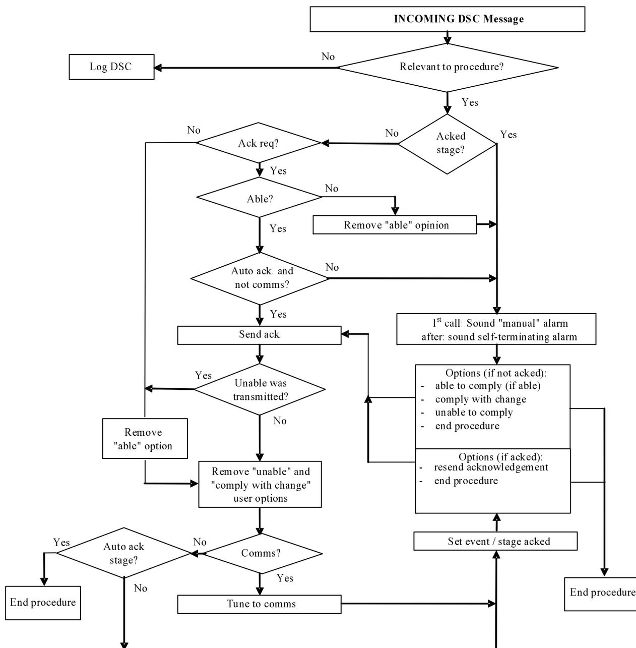
**Figure 8: Receiving non distress procedure**
