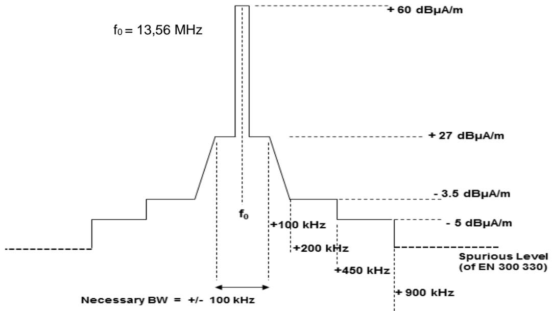
Figure J.4: Spectrum mask limit for narrowband RFIDs in the 13,56 MHz range
