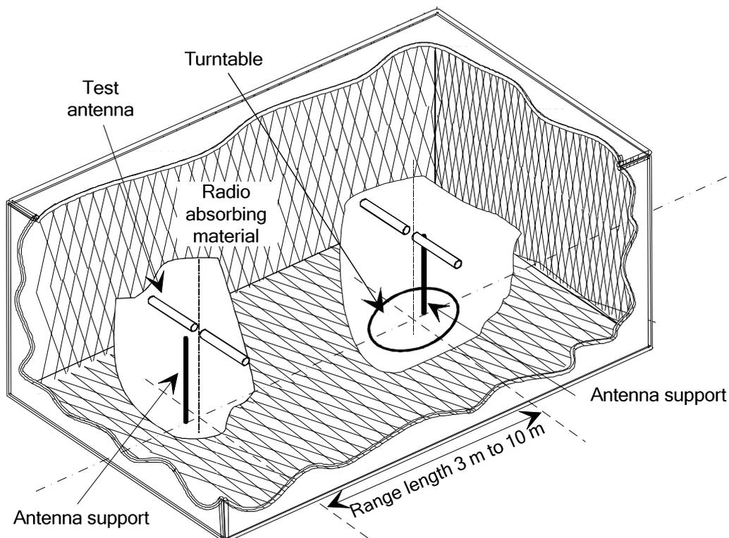
Figure D.1: A typical anechoic chamber
