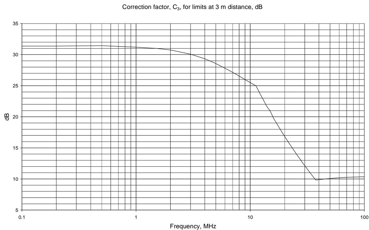
**Figure I.2: Conversion factor  $C_3$  versus frequency**
