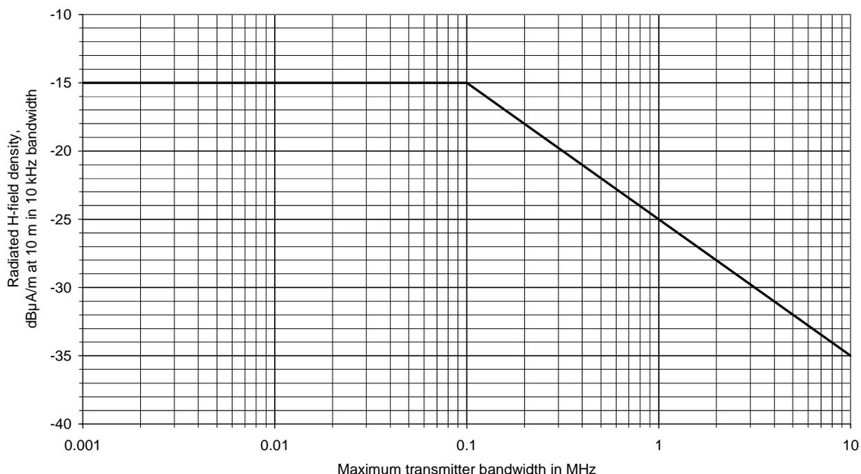
**Figure K.1: Radiated bandwidth and H-field density at 10 m distance**
