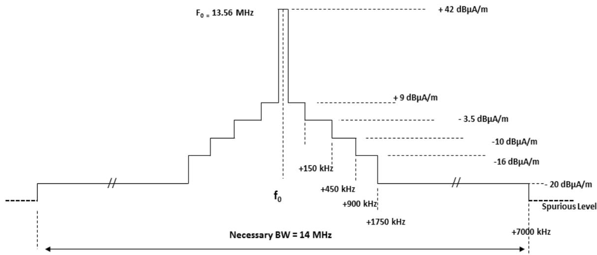
Figure J.3: Spectrum mask limit for wideband RFIDs in the 13,56 MHz range
