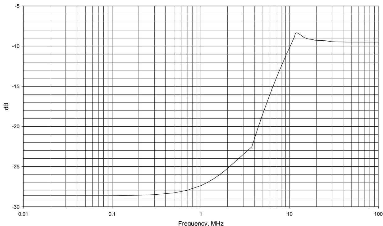
Figure I.1: Conversion factor  $C_{30}$  versus frequency
