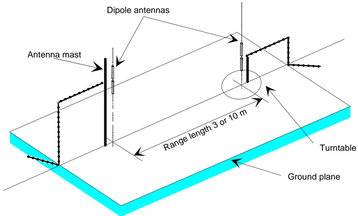
Figure D.3: A typical Open Area Test Site
