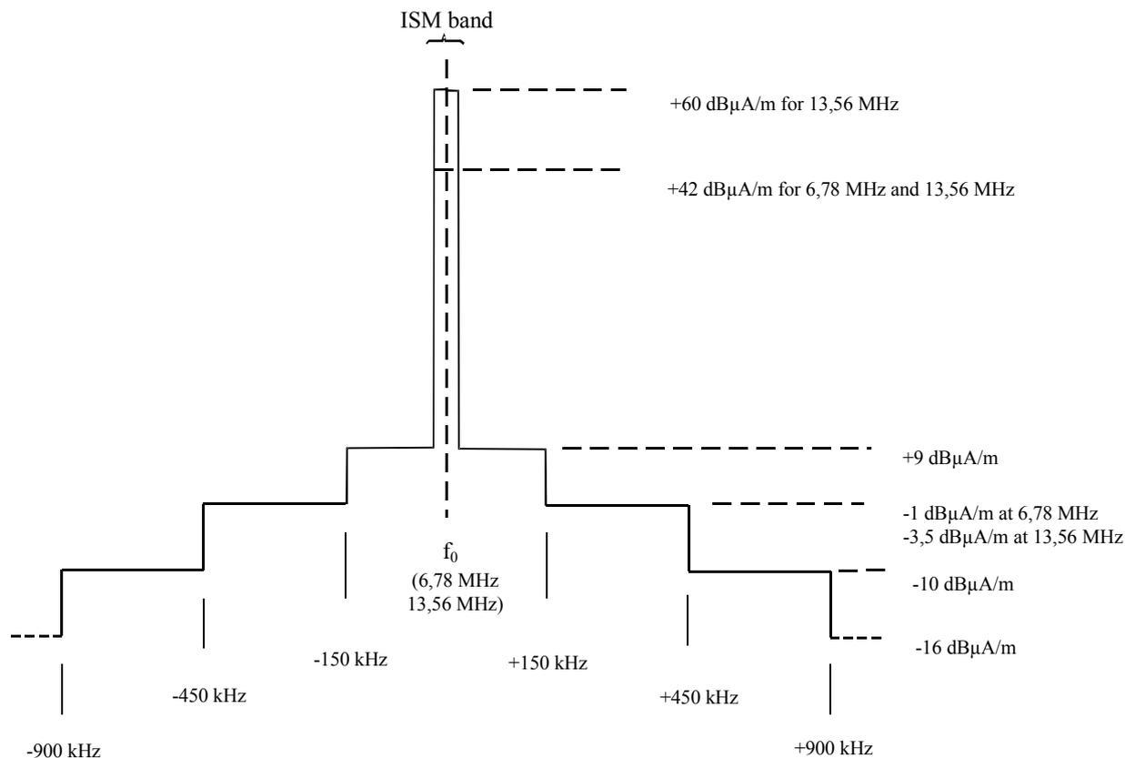
Figure J.2: Spectrum mask limit for RFIDs and EAS in the 6,78 MHz and 13,56 MHz range
