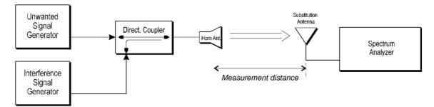
Figure C.3: Measurement Set-up - Calibration
