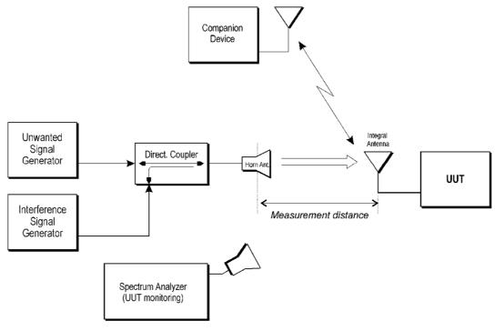
Figure C.2: Measurement Set-up
