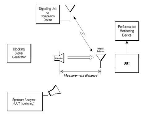
Figure C.4: Measurement Set-up
