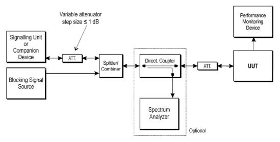
Figure 6: Test Set-up for receiver blocking
