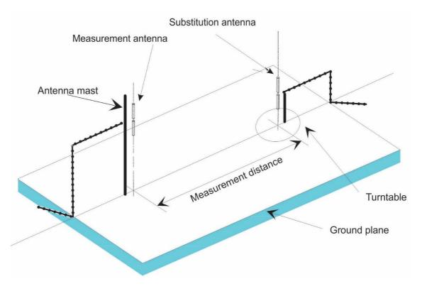
Figure B.1: A typical Open Area Test Site
