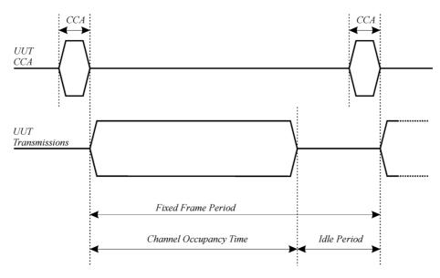
Figure 2: Example of timing for Frame Based Equipment
